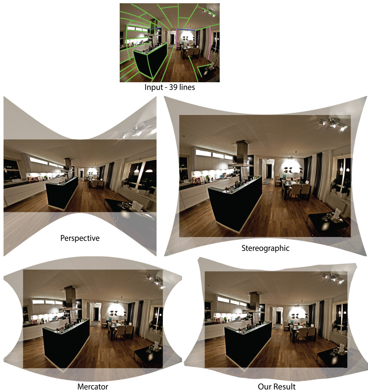
Figure 3.4: We compare the uncropped and manually cropped results of our system to three global projections. The input image was taken from a 140^\circ horizontal field of view fisheye lens. This field of view is well beyond the typical limits for perspective projection, causing severe stretching. The Mercator projection bends the lines between walls and ceiling, and the stereographic projection bends vertical lines. Our result is similar to the conformal projections, but with straight lines.
