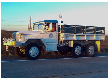
Figure 3.3: FHWA class 6 truck driven on the test section.
