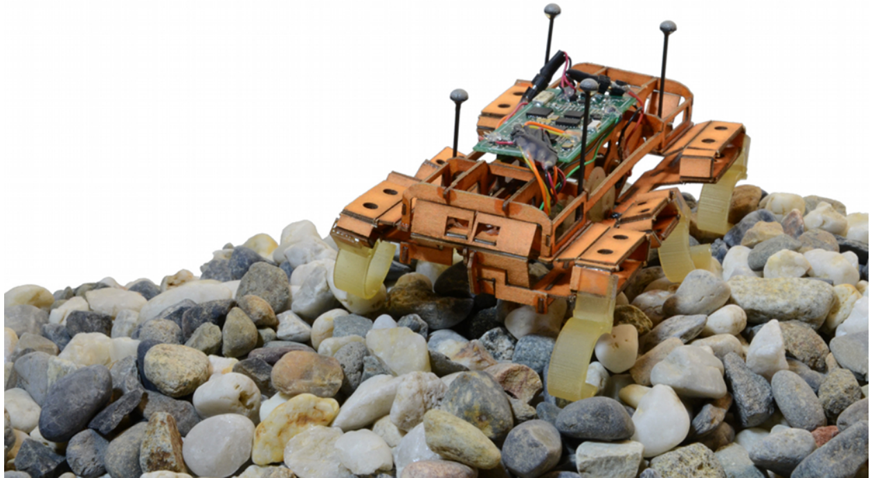
Figure 2.1: VelociRoACH robot, outfitted with motion capture tracking dots, positioned on top of the gravel used for experimentation.
