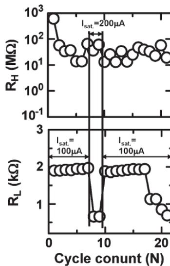
Figure 1.31. The history dependent instability of  $R_{on}$  [55]
