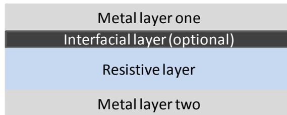
Figure 1.13. basic structure of RRAM
