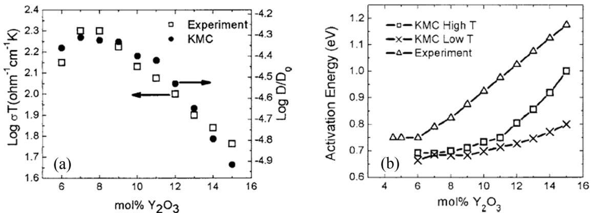
Figure 3.2. (a) The conductivity of YSZ vs the concentration of  $Y_2O_3$  inside  $ZrO_2$  (b) The relationship between the migration energy barrier of  $O^{2-}$  and the concentration of  $Y_2O_3$  [4].
