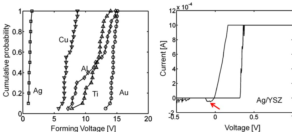
Figure 3.6. (a) The forming voltage distribution for various top electrodes. The device structure I is used. (b) The typical I-V characteristics for Ag/YSZ device. The red arrow shows the very small  $V_{\text{RESET}}$
