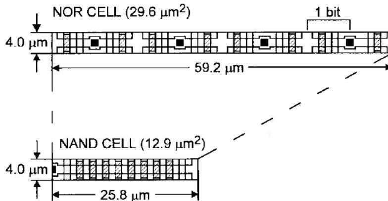
Fig. 1.10. Layout comparisons between NAND and NOR Flash [12].
