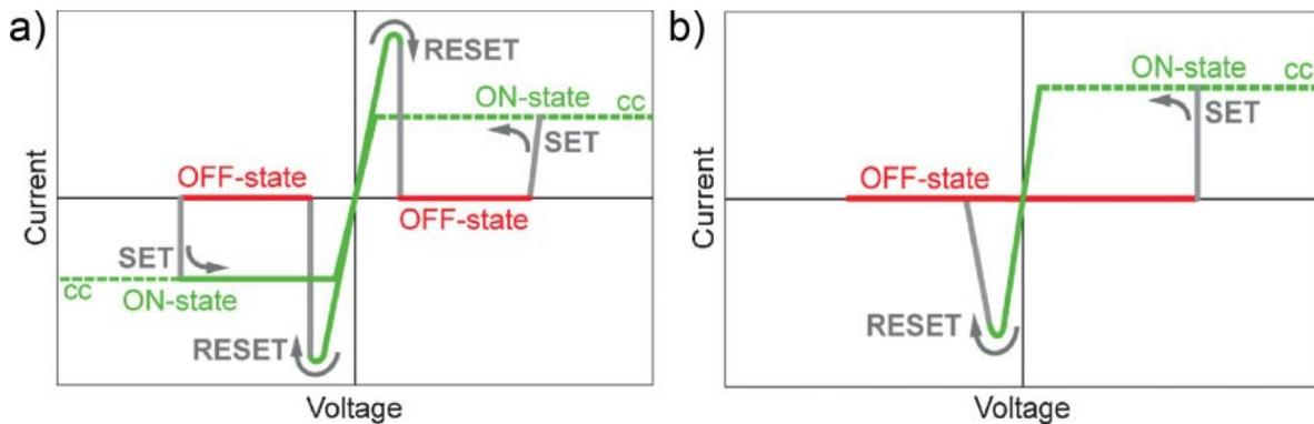
Figure 1.14. Two operation schemes for RRAM (a) unipolar device (b) bipolar device [25]
