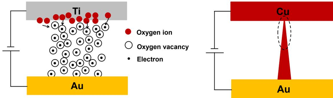
Figure 4.3. The filament width comparison between Ti/YSZ and Cu/YSZ in RESET stage.
