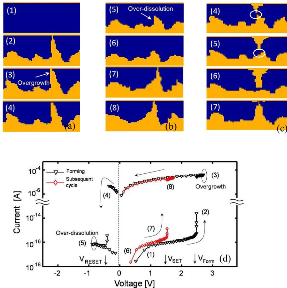
Figure 2.18. KMC Simulated I-V characteristics and related filament topographies (for the first scenario). The voltage sweep rate is 1V/s. Simulation starts from (1) and ends at (8). All the critical physical parameters are indicated in the figures. Overgrowth and over-dissolution are clearly seen And  $V_{\text{SET}}$  in the subsequent cycle is much less than  $V_{\text{Form}}$ . The external resistance is set to 30k $\Omega$ . Filament resistivity is  $5 \times 10^{-6} \Omega\text{m}$
