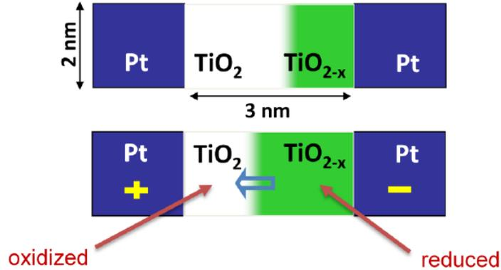
Figure 1.21. switch mechanism of Pt/TiO<sub>2</sub>/Pt cell [2]
