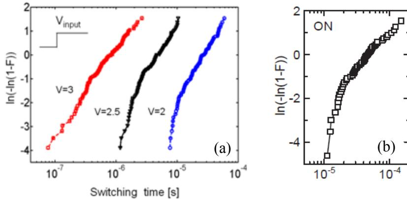
Figure 2.15. (a) Simulated switching time  $t_{ON}$  distribution under different input conditions (b) experimental results in Cu/Ta<sub>2</sub>O<sub>5</sub> system [10].
