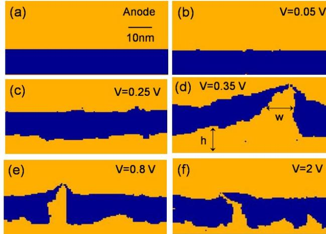
Figure 2.7. Filament topographies obtained at different voltage levels. (a) initial state. (b)  $V=0.05$  V. (c)  $V=0.25$  V. (d)  $V=0.35$  V. (e)  $V=0.8$  V. (f)  $V=2$  V. The arrows in (d) with labels 'h' and 'w' indicate the thickness of isotropic deposition and the average width of the filament respectively [4, 7].
