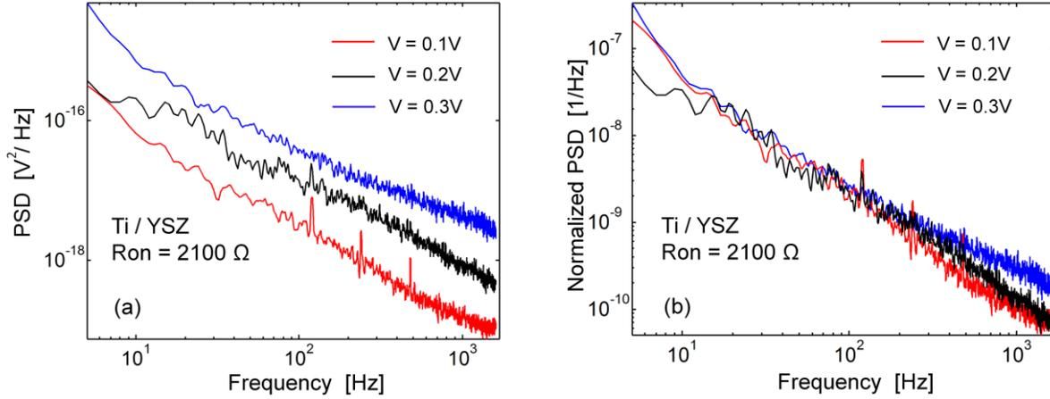
Figure 3.21. (a) The noise power spectrum density and (b) normalized PSD of Ti/YSZ at the resistance state of 2100Ω.
