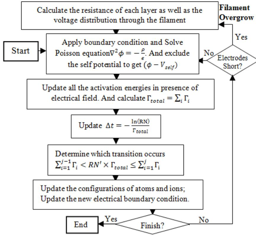
Figure 2.6. The flowchart of the KMC simulation process. RN and RN' are random numbers uniformly distributed between [0 1]
