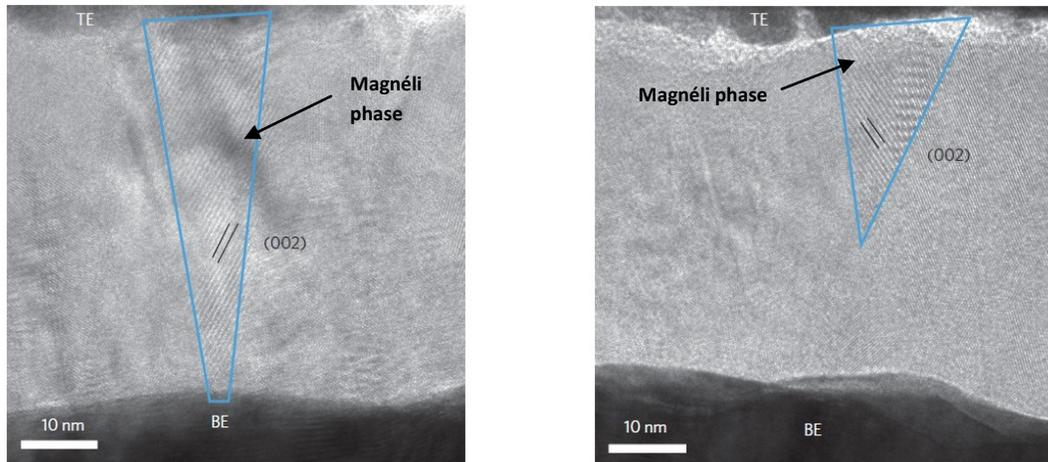
Figure 1.26. TEM image of Magnéli phase after the forming process inside of Pt/TiO<sub>2</sub>/Pt cell (Left) and a discontinued Magnéli phase (Right) [44]
