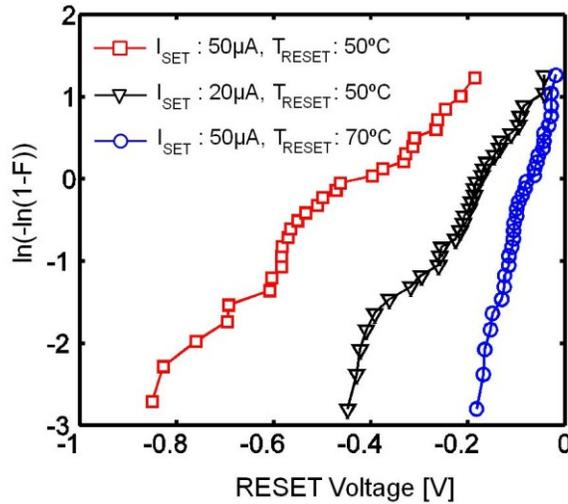
Figure 2.19.  $V_{\text{RESET}}$  distribution at different SET control current and RESET temperature levels.
