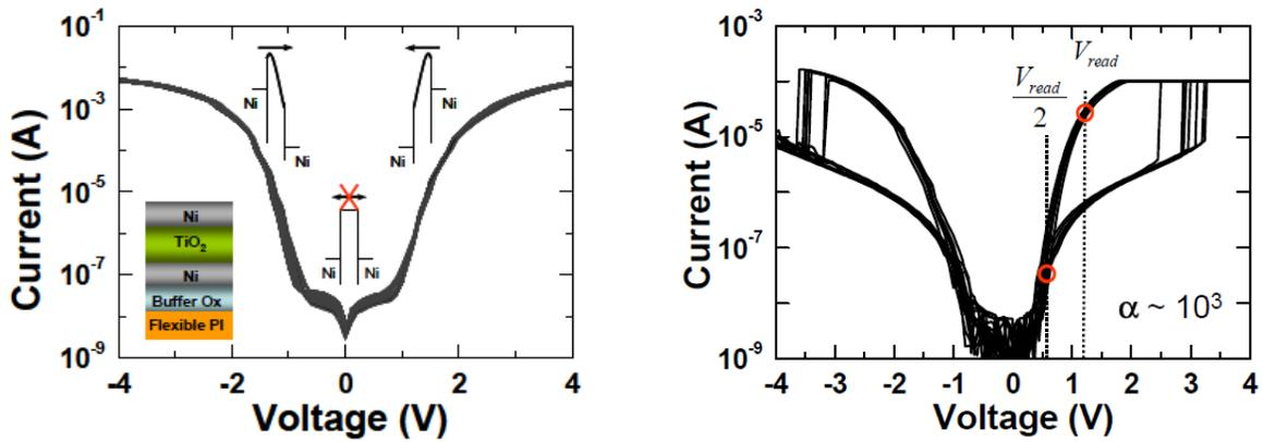
Figure 1.29. A bidirectional selector based on Ni/TiO<sub>2</sub>/Ni (left) and the overall performance of a bidirectional selector integrated with Ni/HfO<sub>2</sub>/Pt RRAM (right) [51]
