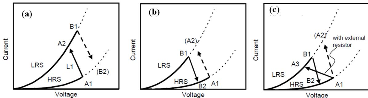
Figure 1.19. Several switching modes in unipolar RRAM (a) stable SET (b) stable RESET (c) both stable SET and RESET [33]
