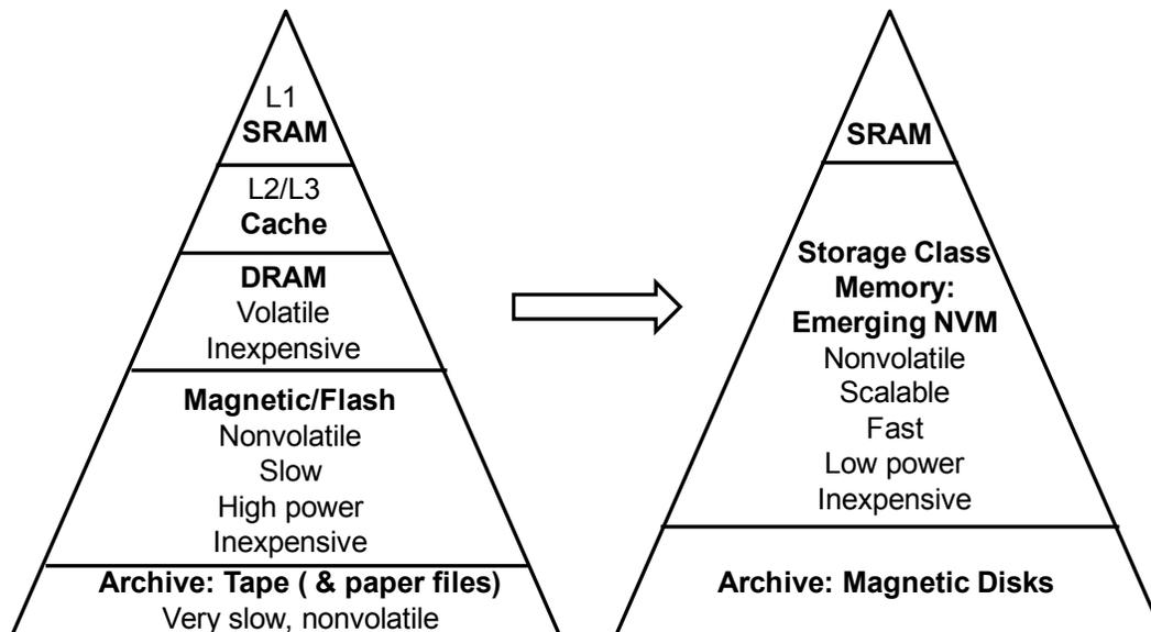
Figure 1.12. The modification of memory hierarchy upon realization of a universal memory (storage class memory) [18]
