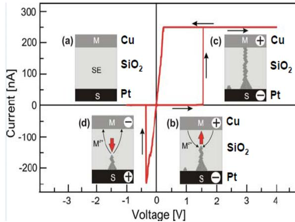
Figure 1.15. I-V characteristics of Cu/SiO<sub>2</sub>/Pt [26]
