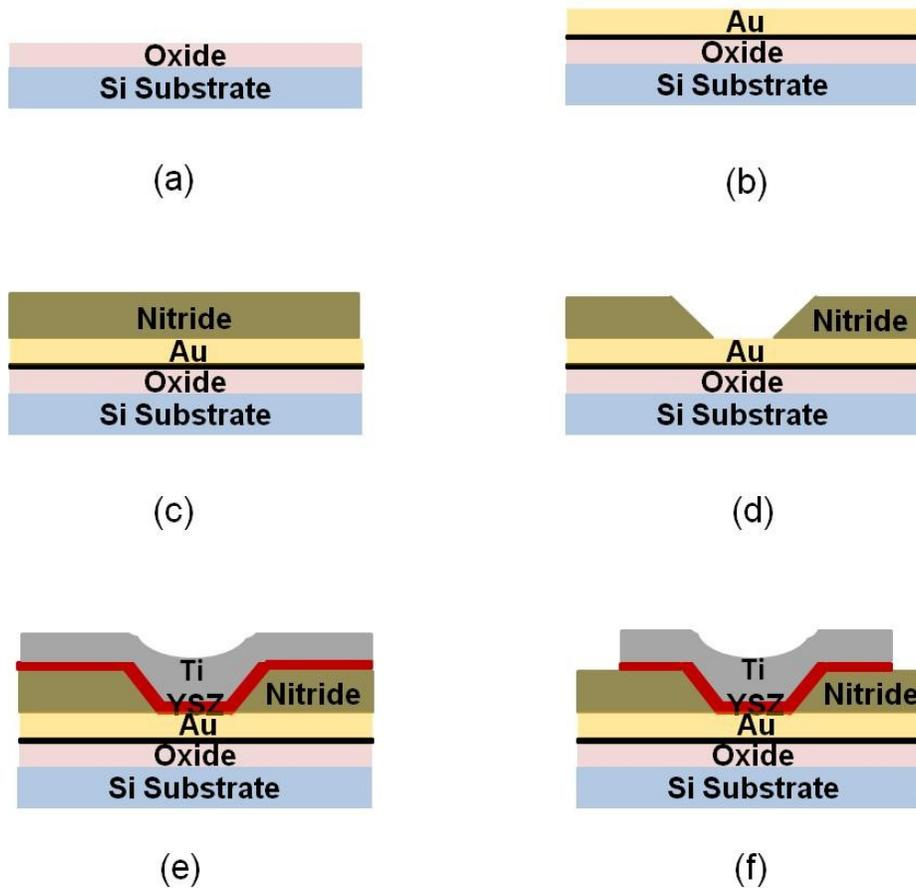
Figure 3.5. Experimental procedures for device structure II
