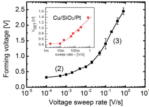
Figure 2.10. Simulated  $V_{\text{Form}}$  vs voltage sweep rate [4, 7]. The inset shows the experimental results on Cu/SiO<sub>2</sub>/Pt system [9]
