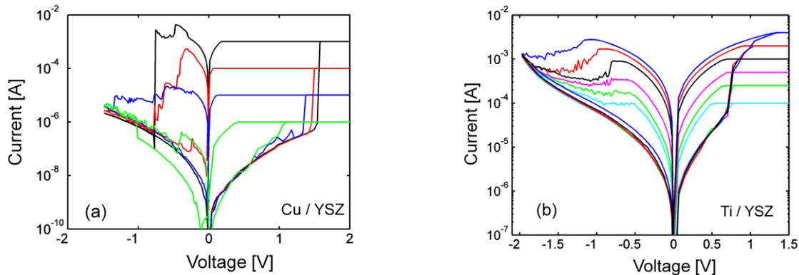
Figure 3.9. The I-V characteristics of (a) Cu/YSZ and (b) Ti/YSZ at different current compliance levels. YSZ film thickness is 10nm. Device area is 16um by 16um.
