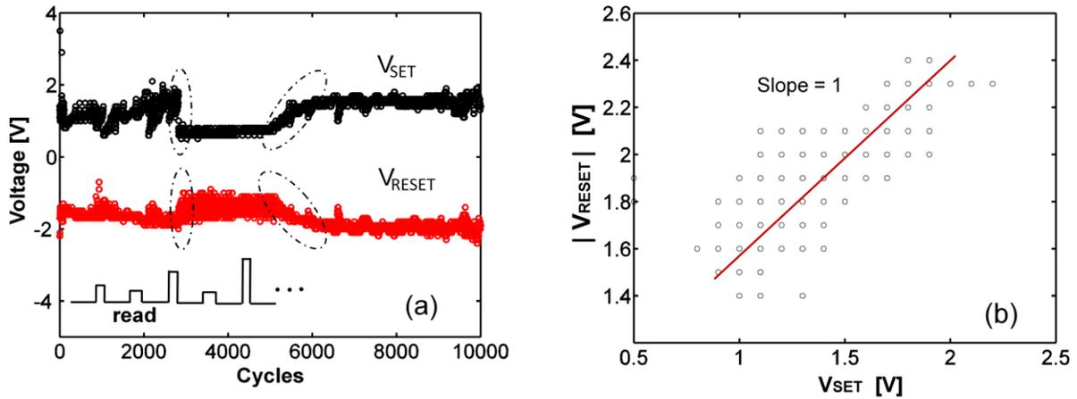
Figure 4.5. (a) The Evolution of  $V_{\text{SET}}$  and  $V_{\text{RESET}}$ . The dash line shows both a sudden and a gradual change in  $V_{\text{SET}}$  and  $V_{\text{RESET}}$  (b) The relationship between  $V_{\text{SET}}$  and  $V_{\text{RESET}}$  for an endurance test of  $10^4$  cycles.
