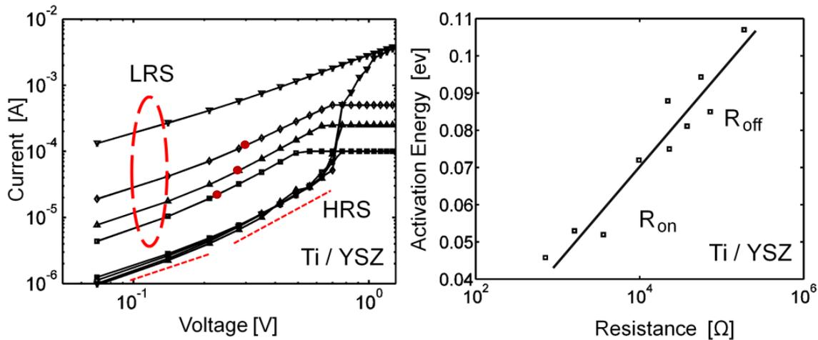
Figure 3.13. (a) The SET stage I-V of Ti/YSZ . The dashed lines indicate slopes of 1 and 2 respectively (b) Extracted activation energy at different resistance levels
