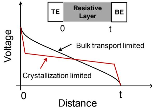
Figure 1.20. The voltage distribution across the resistive layer in bulk transport limited and crystallization limited cases
