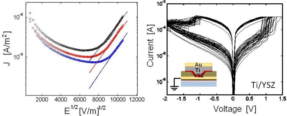
Figure 3.8. (a) Experimental (symbols) and simulated (lines) results of the forming stage I-V for Ti/YSZ. The measurements are taken at 30°C, 50°C and 70°C respectively. (b) 300 repetitive I-V sweeps for a typical Ti/YSZ device (The sweep count was limited by practical measurement time). YSZ film thickness is 10nm. Device area is 16µm by 16µm.
