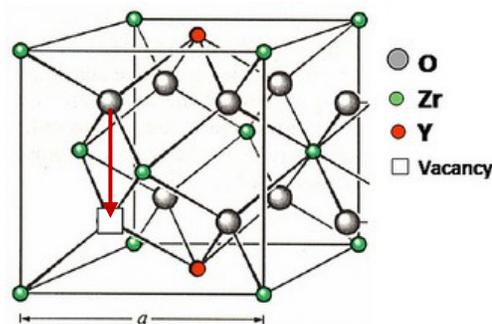
Figure 3.1. The crystal structure of YSZ [3]
