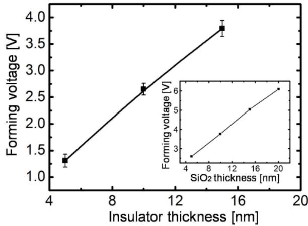
Figure 2.11. Simulated  $V_{\text{Form}}$  vs. insulator layer thickness. The sweep rate is 1V/s. Inset shows experimental result for Cu/SiO<sub>2</sub>/Pt system [9].
