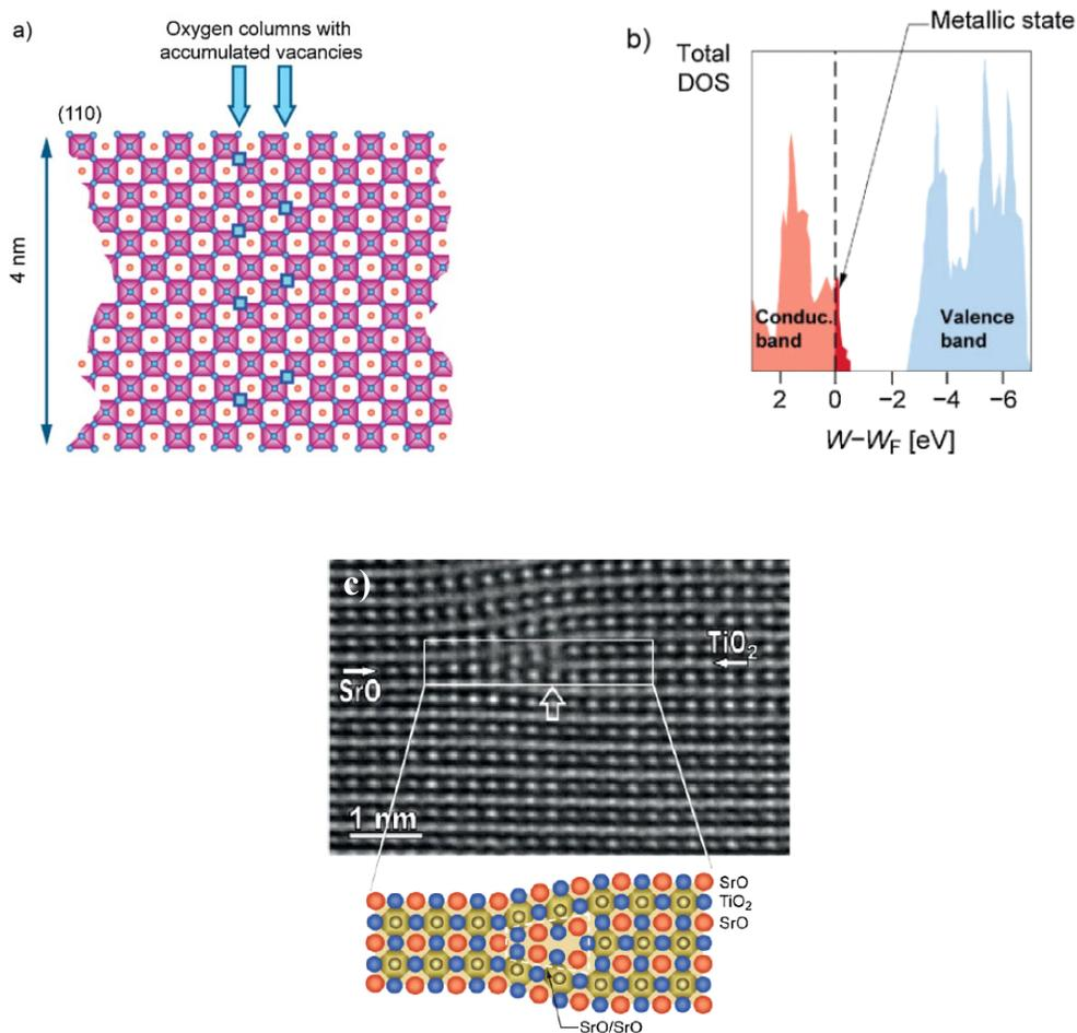
Figure 1.25. (a) The VO accumulation along lines in SrTiO<sub>3</sub> [25] [41] (b) Calculated density of states close to the defect region [18] (c) Illustration of lattice structure close to the core of edge dislocations in SrTiO<sub>3</sub>[25] [42].
