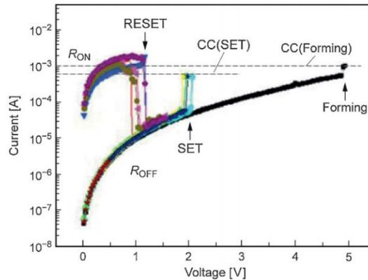
Figure 1.16. I-V characteristic of a Pt/NiO/Pt stack [28]
