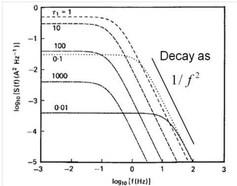
Figure 3.20. Lorentzian power spectra calculated based on Equation 13 [26]
