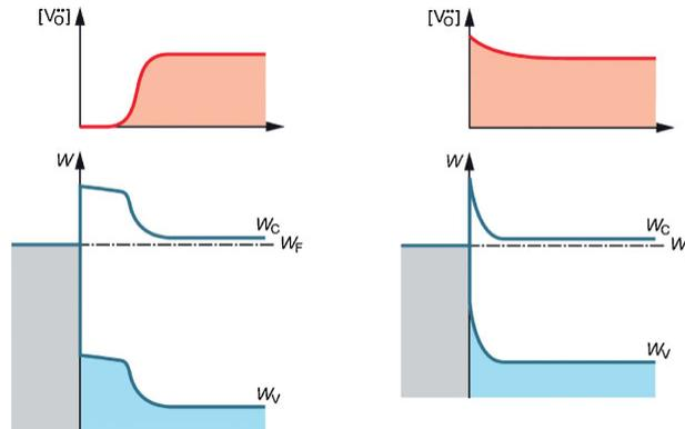
Figure 1.22. The VO distribution and the band diagram for Pt/TiO<sub>2</sub>/Pt system [25]
