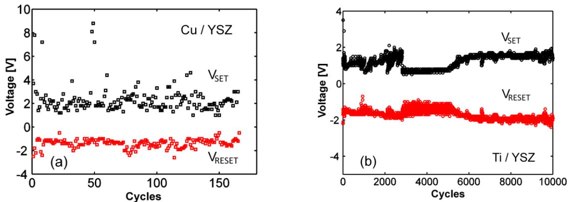
Figure 3.16. SET and RESET voltage distribution for Cu/YSZ (a) and Ti/YSZ device (b)
