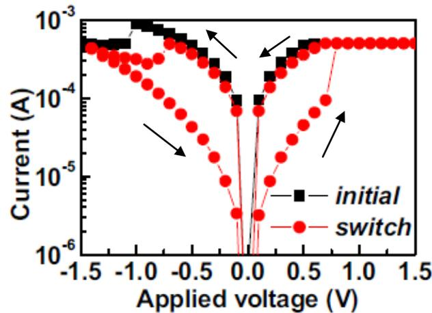
Figure 1.24. The I-V characteristics of a Ti/HfO<sub>2</sub>/TiN stack [40]
