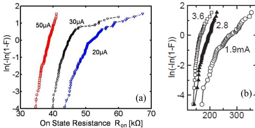
Figure 2.16. (a) Simulated on-state resistance distribution under different current input conditions (b) the experimental results for the Cu/Ta<sub>2</sub>O<sub>5</sub> system [10]
