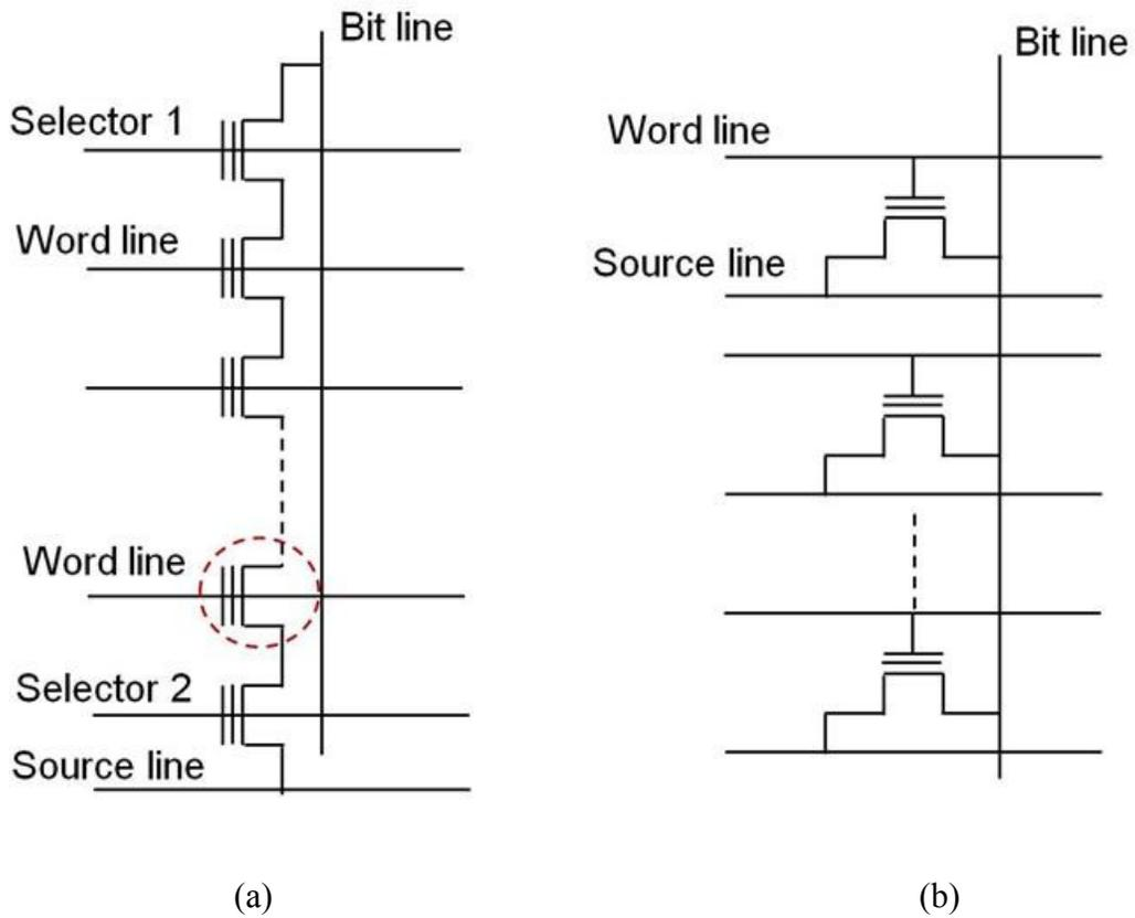
Figure 1.9. (a) The NAND array structure of FLASH (b) the NOR array structure.
