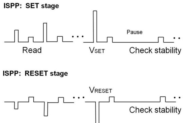
Figure 3.14. The incremental step pulse programming methodology
