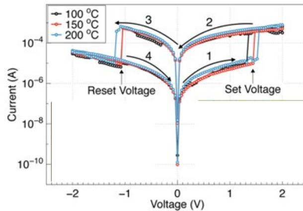
Figure 1.18. I-V characteristic Ag/Ag<sub>2</sub>Se/Pt stack [29]
