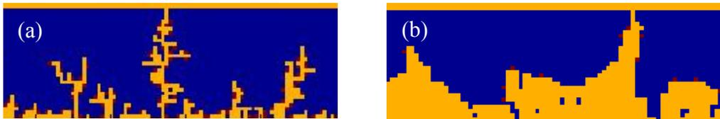
Figure 2.20. Simulated Filament shape formed under different conditions. (a) when the activation energy  $E_{\text{surf}}$  is large while  $E_{\text{adatom}}$  is small (b) when  $E_{\text{surf}}$  is small and  $E_{\text{adatom}}$  is large.
