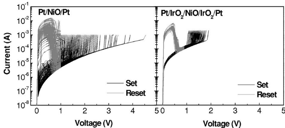
Figure 3.17. I-V characteristics of Pt/NiO/Pt stack (left) and Pt/IrO<sub>2</sub>/NiO/IrO<sub>2</sub>/Pt stack [21].
