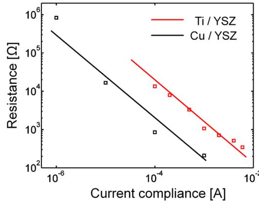
Figure 3.10. The relationship between  $R_{on}$  and current compliance for both Cu/YSZ and Ti/YSZ
