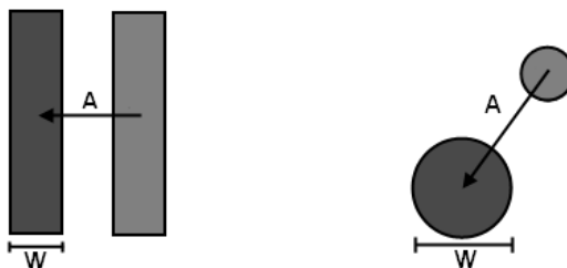
Figure 2.2. Using a Java applet, sequences of rectangular and circular targets are presented, where target distance A and width W can remain constant (homogeneous) or vary (heterogeneous) after every click.
