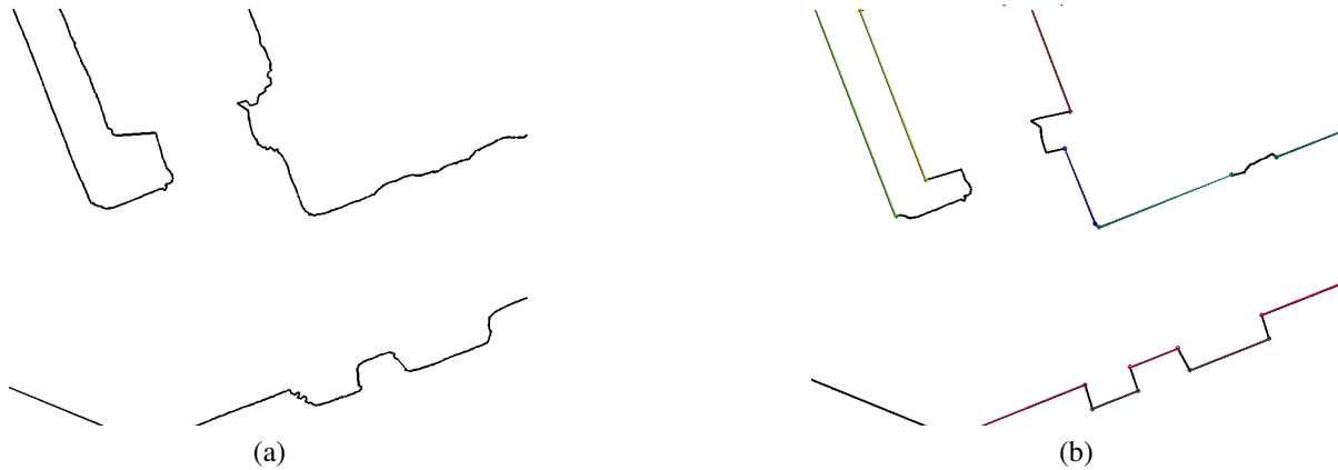
Figure 8. (a) Watertight wall edges; (b) curve-fitting via RANSAC reduces sample location error and sharpens corners.
