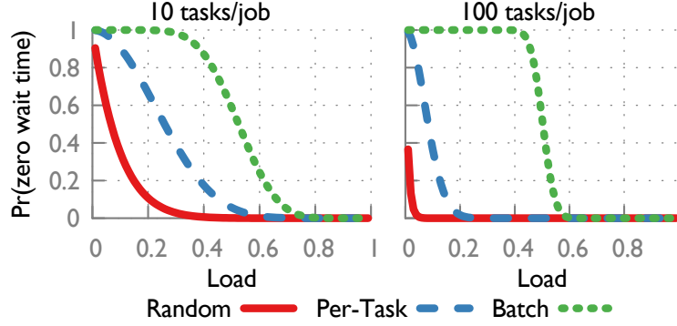
Figure 4: Probability that a job will experience zero wait time in a single-core environment, using random placement, sampling 2 servers/task, and sampling 2m machines to place an m -task job.
