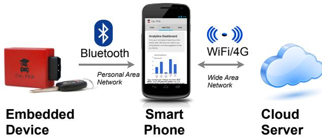
Figure 1. An example MPC application distributes logic and user interaction across embedded device, mobile phone and a cloud server.
