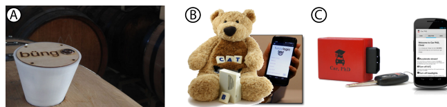
Figure 4. Example devices from our class: A) A wireless barrel gauge for distilleries and wineries; barrel readings are aggregated online. B) A toy to support literacy education; play statistics are collected on the phone and online. C) A car dongle that streams driving telemetry data to the phone and compares driving behavior on a central server.
