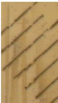
Figure 3.12 Micrograph of the gravure printed organometallic silver ink.
