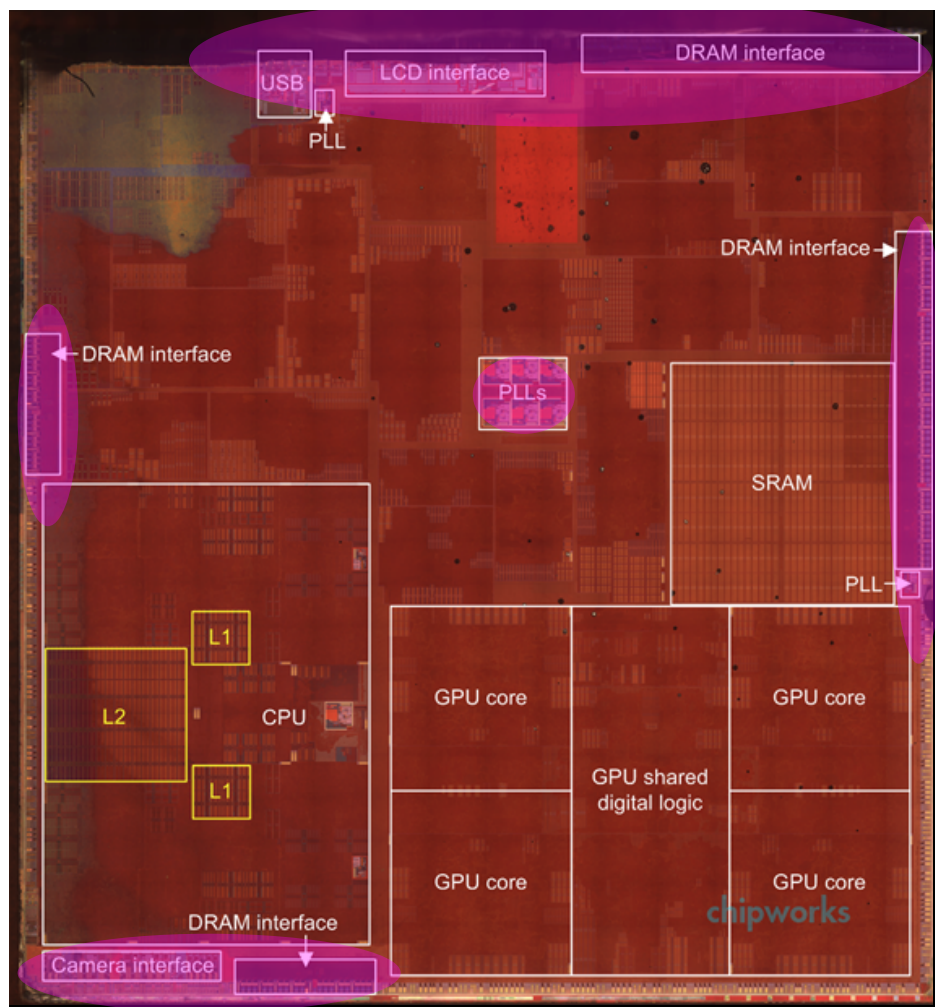
Figure 1.1: Apple A7 SoC with some of the AMS blocks highlighted [2].
