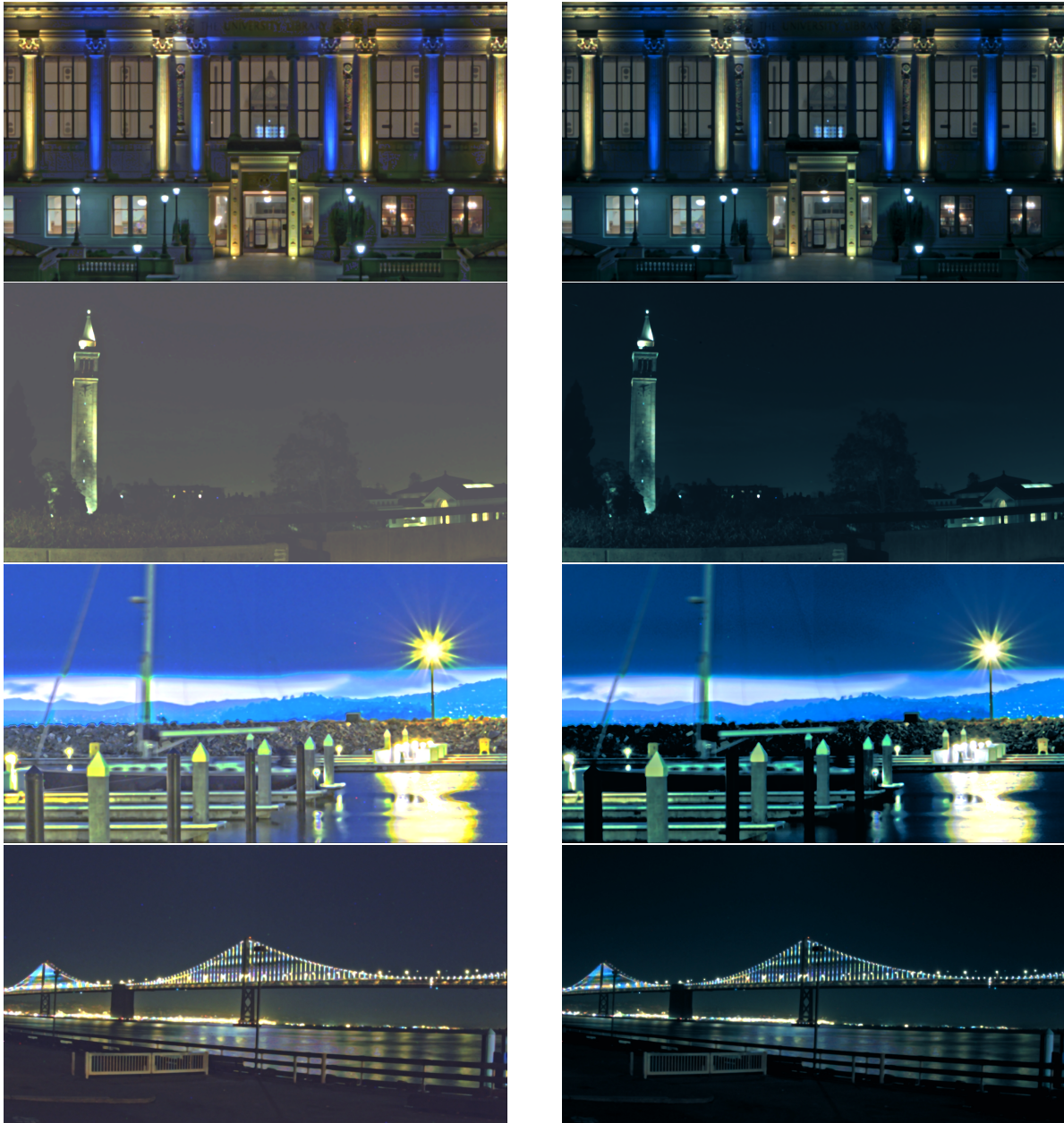
Figure 12: (Left) Images generated without modeling the Purkinje effect or the perceptible illumination interval. (Right) Images generated with our method. We did not perform any color correction or additional processing other than using the algorithm described in this paper.
