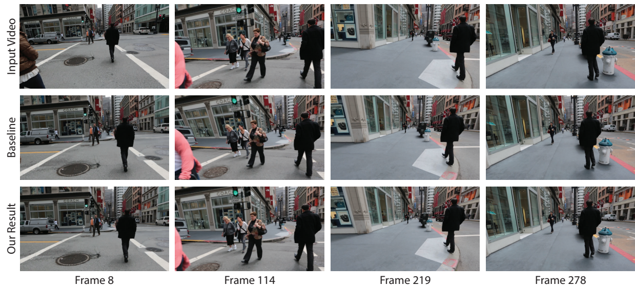
Figure 5.13: The suddenly jerk in the video at frame 114 results in the left facade being heavily distorted in the baseline stabilization. Notice how our result reduces the distortion.
