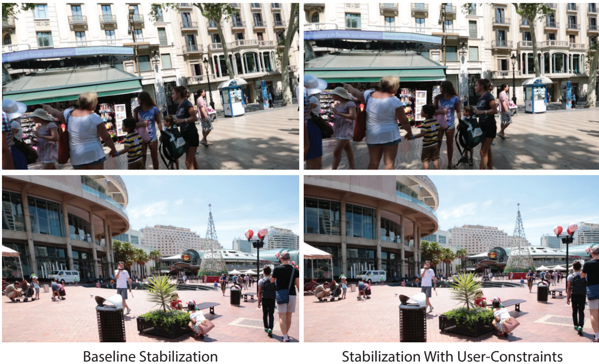
Figure 5.9: Comparison of initial baseline with result using user constraints. In all examples on the left, the baseline stabilization is not satisfactory as the scene is distorted and the horizon is not level. The same frames in our result are less distorted as the structures are vertical.
