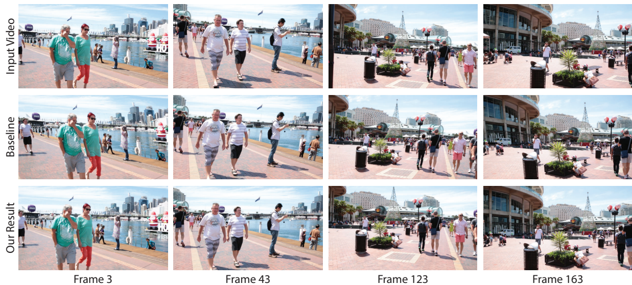
Figure 5.15: Notice how subjects and faces in the baseline results are skewed in either direction due to the extreme shake of the camera. In our result, these distortions are more pleasing to the eye as structures are largely vertical and pedestrians are not skewed.
