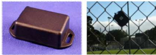
Figure 2.3: The IP-65 enclosure (rain and dust resistant) that houses the hardware platform [courtesy of Hammond Inc] shown next to one sensor as deployed in the middle of a fence section
