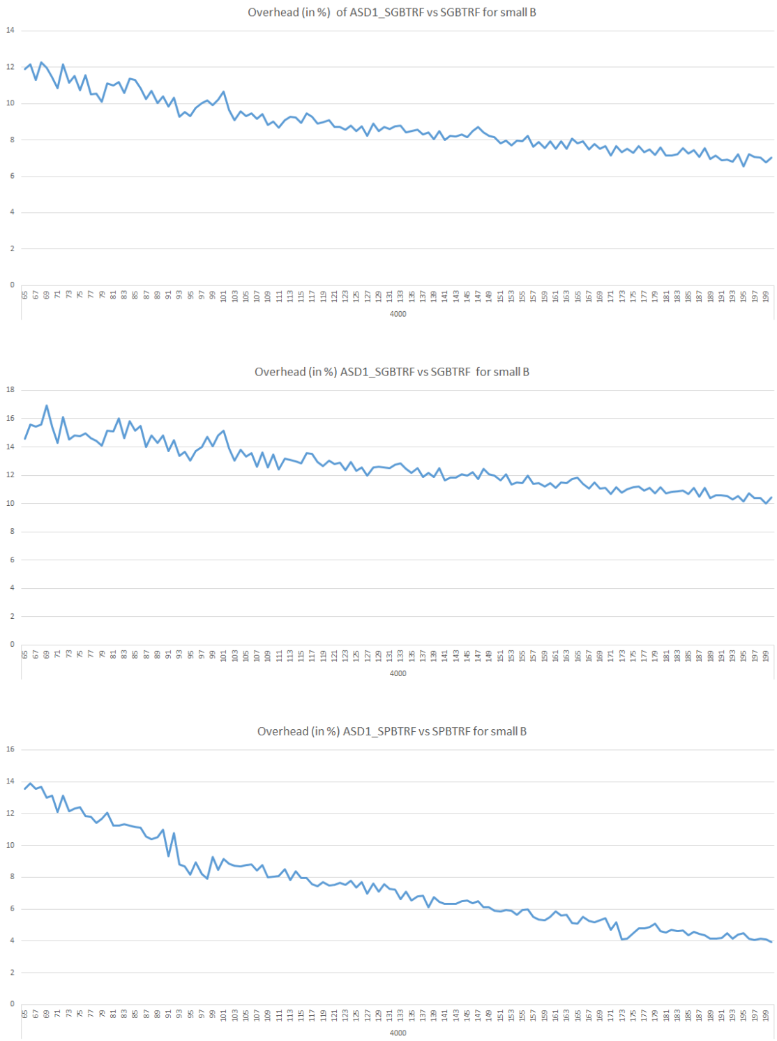
Figure 5.6. Small b overhead for Top : ASD1_SGBTRF on random matrix (with pivoting) Middle : ASD1_SGBTRF on random Positive Definite matrix (without pivoting) Bottom : ASD1_SPBTRF on random Positive Definite matrix
