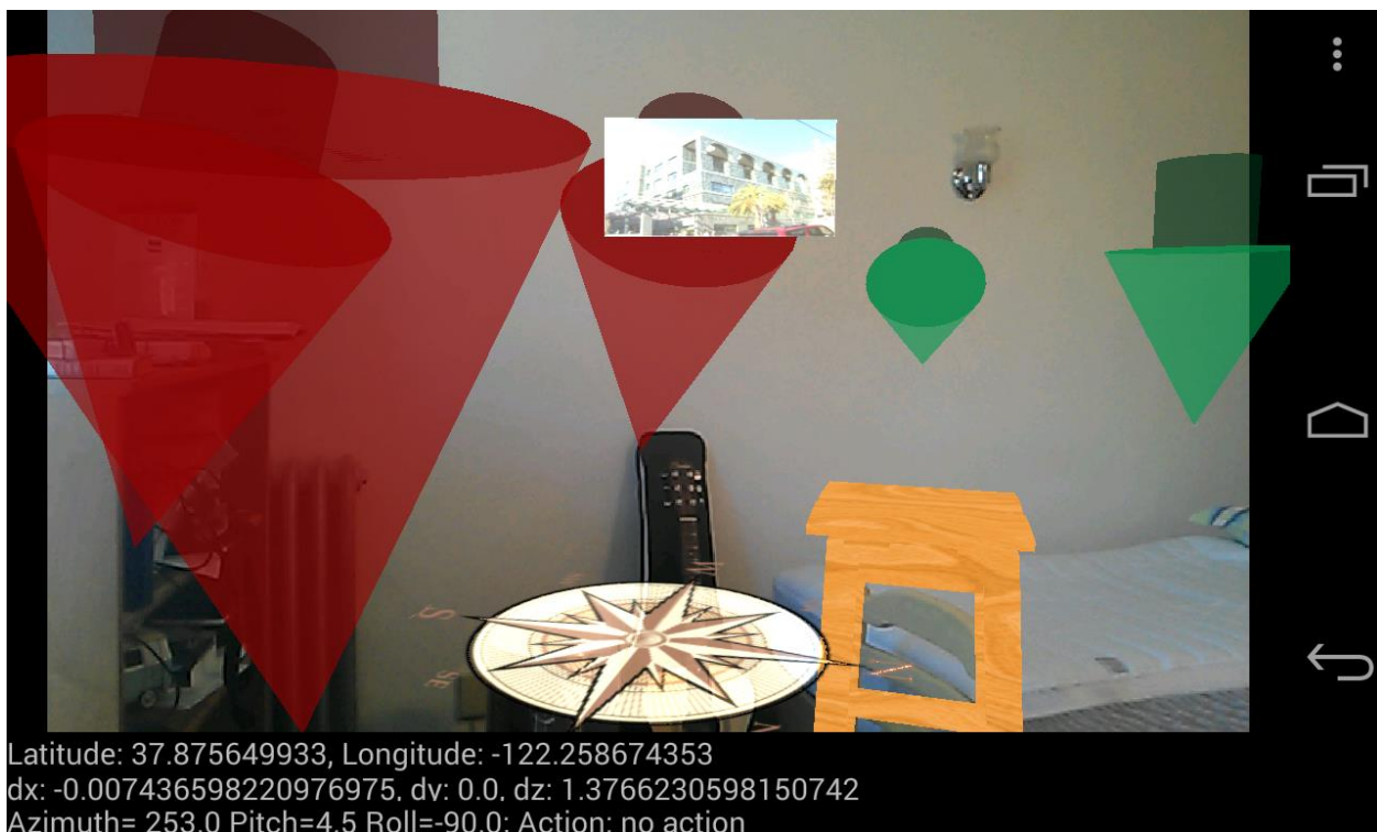
Figure 10. Graphics layer made of rectangular textures, 3D textured objects (chair) and non-textured arrows
