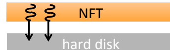
Figure 19: A summary of the various energy transfer methods in the HAMR NFT, air gap and hard disk. The most dominant energy transfers are via near-field light coupling from NFT to disk, heat conduction through the high-conductivity NFT and heat-conduction into the large hard disk substrate.
