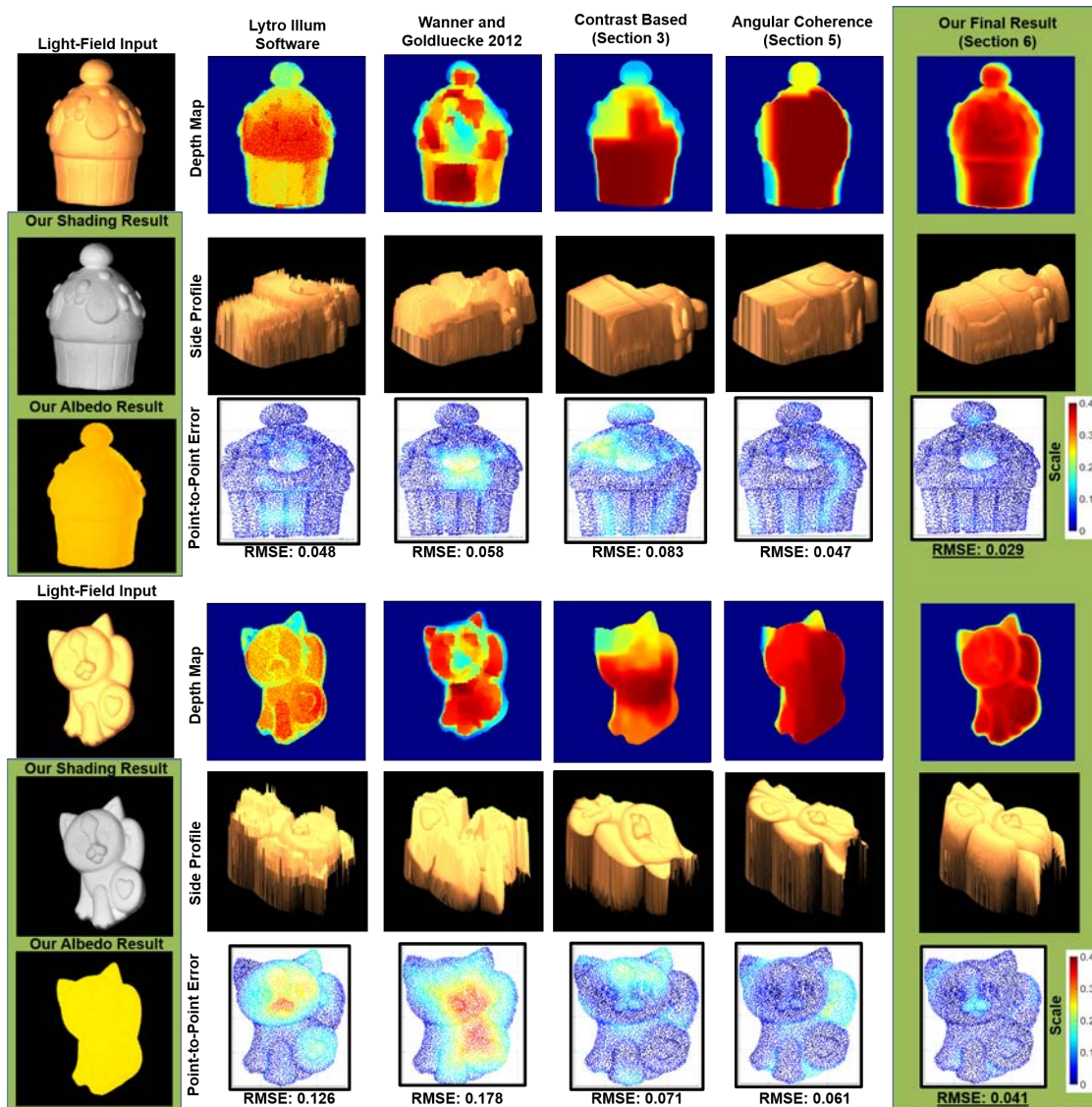
Figure 3.10: Uniform Albedo Comparisons. We compare qualitative and quantitative measures with two different examples against Lytro Illum Software, Wanner and Goldluecke [83], contrast-based defocus and correspondence from Chapter 3.3, and angular coherence based defocus and correspondence from Chapter 3.5. On the top, we have an example of a cupcake, where our algorithm is able to estimate the contours of the cupcake decorations. On the bottom, we have an image of a flat cat figurine. We can see that our algorithm is able to recover the curvature of the body and face. For comparison against ground truth, we use the NextEngine 3D scanner to obtain the ground truth and align each of the resulting depth maps using the iterative closest point (ICP) algorithm. The color diagram shows the Euclidean distance of each ground truth point to the closest point after the ICP transformation for each algorithm. We can see that we align closely with the ground truth with the lowest RMSE.
