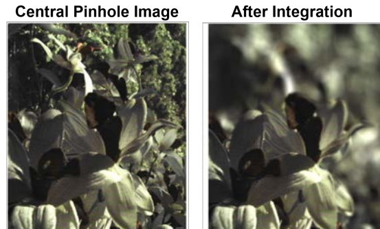
Figure 2.7: Refocusing. On the left, we only use the central viewpoint to generate the output image. By integrating a small 7 \times 7 angular pixel neighborhood, we show that we decrease the depth-of-field significantly.
