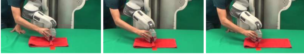
Figure 3.3: Demonstrations of folding the towel using the red tape as reference for the target fold.
