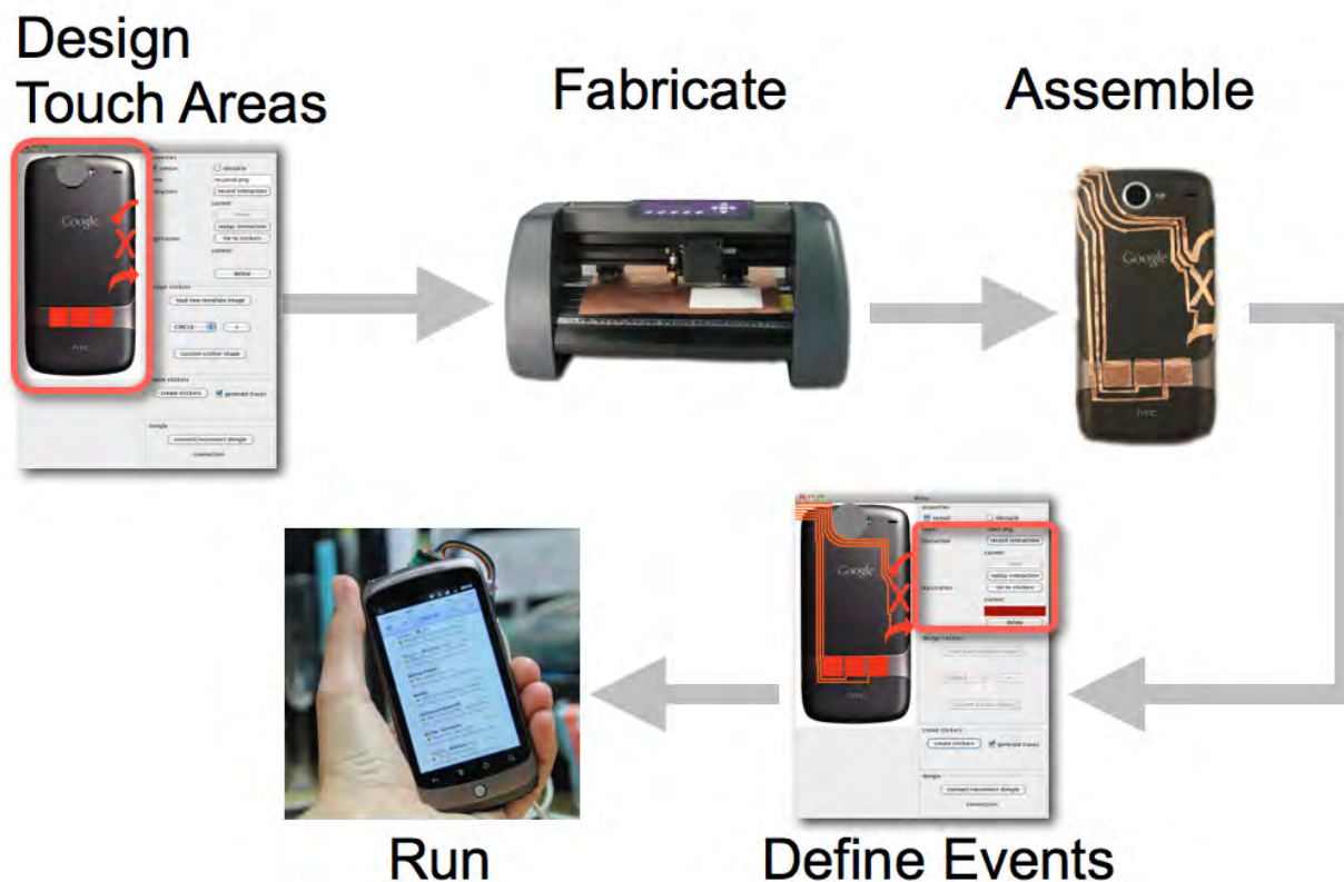
Figure 4.1: Midas enables users to define discrete and continuous touch sensors with custom shapes and layout. It generates fabrication files and assembly instructions. Designers can also define the interaction events of their prototype.
