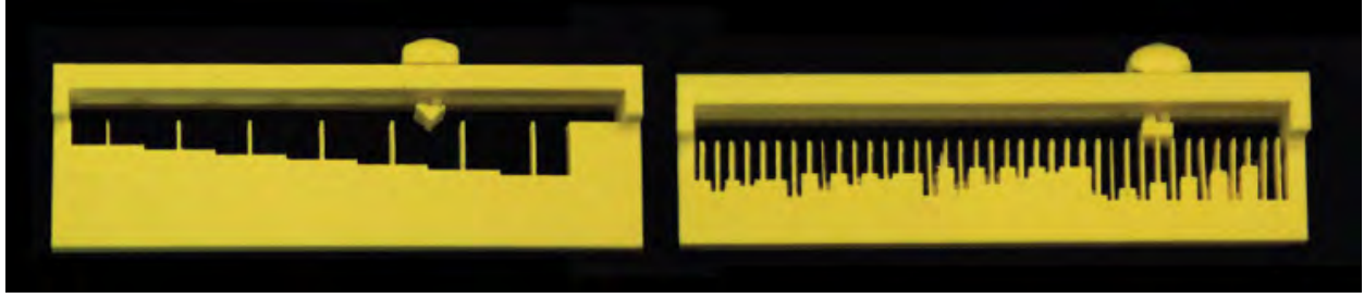
Figure 5.5: We experimented with two different encoding mechanisms for sliders: linearly increasing sequences (left) and de Bruijn (right). de Bruijn sequences allow classification of fewer tine lengths, but require more consecutive tine recognitions to determine position and direction.
