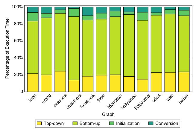
Figure 3.14: Categorization of execution time by hybrid-heuristic
