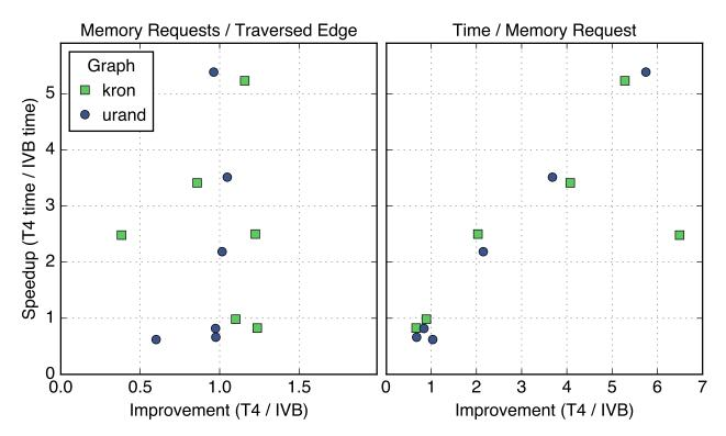
Figure 6.5: Speedup of IVB over T4 versus IVB's improvement over T4 in GAIL metrics (memory requests per traversed edge versus inverse memory bandwidth) for GAP benchmark kernels processing the kron and urand graphs.
