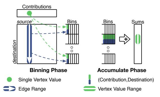
Figure 7.4: Propagation blocking. In the binning phase, vertices pair their contributions with their destination indices and insert them into the appropriate bins. In the accumulate phase, the contributions are reduced into the correct sums.
