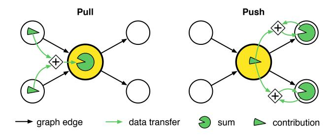
Figure 7.1: PageRank communication for pull direction (left) and push direction (right). In the pull direction, the active vertex (shaded) reads the contributions of its incoming neighbors and adds them to its own sum. In the push direction, the active vertex adds its contribution to the sums of its outgoing neighbors.
