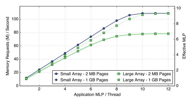
Figure 5.4: Impact of 2 MB and 1 GB page sizes on memory bandwidth achieved by single-thread parallel pointer chase for array sizes of *small* (1 GB) and *large* (16 GB).
