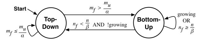
Figure 3.7: Finite-state machine to control the direction-optimizing algorithm. When transitioning between approaches, the frontier must be converted from a queue (top-down) to a bitmap (bottom-up) or vice versa. The *growing* condition indicates the number of active vertices in the frontier  $(n_f)$  increased relative to the last depth.
