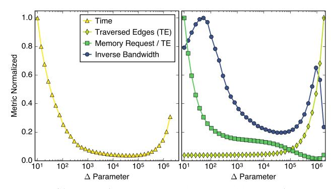
Figure 6.2: GAIL metrics for delta-stepping implementation while varying  $\Delta$ -parameter traversing the road graph using 8-cores on the IVB platform. From the GAIL metrics, we see the U-shape in execution time is caused by the L-shape of the number of memory requests per traversed edge and the backwards L-shape for the number of traversed edges.
