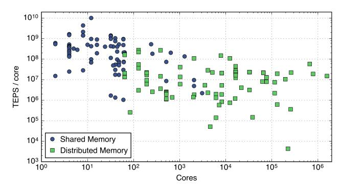
Figure 1.1: Performance per core versus core count for June 2015 Graph 500 rankings [66]. Performance measures traversed edges per second (TEPS) executing breadth-first search.
