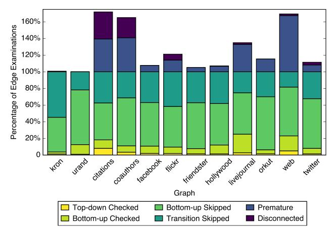
Figure 3.13: Categorization of edge examinations by hybrid-heuristic
