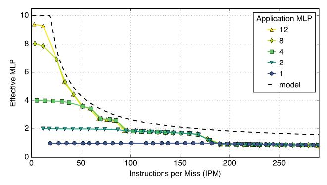
Figure 5.3: Memory bandwidth achieved by parallel pointer chase microbenchmark with varying number of nops inserted (varies IPM). Using a single thread with differing numbers of parallel chases (application MLP).
