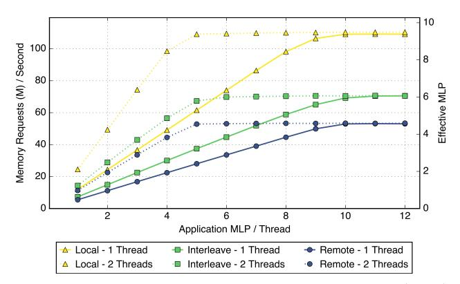
Figure 5.2: Memory bandwidth achieved by parallel pointer chase microbenchmark (random) in units of memory requests per second (left axis) or equivalent effective MLP (right axis) versus the number of parallel chases (application MLP). Single core using 1 or 2 threads and differing memory allocation locations (local, remote, and interleave).
