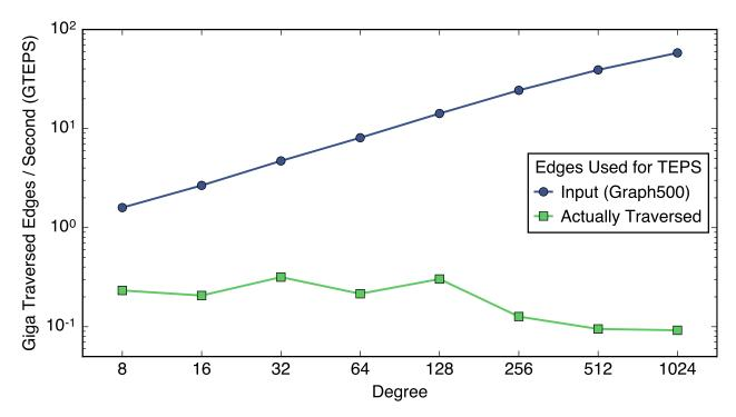
Figure 6.1: Impact of calculating TEPS based on input edges or actual edges traversed when scaling the degree of a 8 million vertex synthetically-generated Kronecker graph. Uses GAP direction-optimizing BFS implementation executing on IVB.
