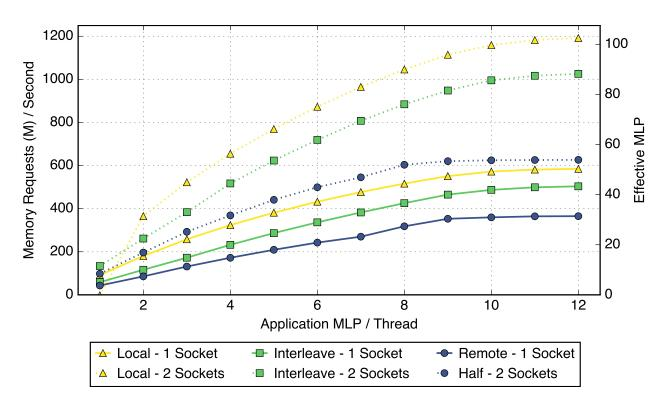
Figure 5.5: Random bandwidth of a socket or the whole system with different memory allocations.
