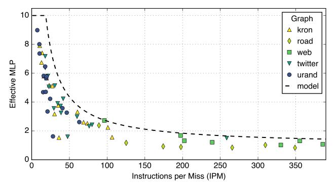
Figure 5.8: Single-thread achieved memory bandwidth of full workload relative to instructions per miss (IPM). Note: Some points from road & web not visible due to IPM>1000 but model continues to serve as an upper bound.
