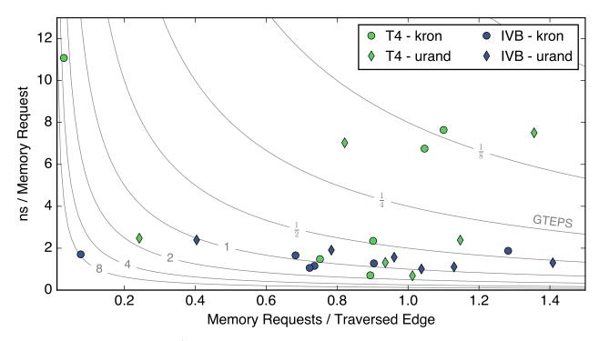
Figure 6.4: GAIL metrics (memory requests per traversed edge versus inverse memory bandwidth) for GAP Benchmark kernels executing on IVB and T4 to process the kron and urand graphs. Contours show GTEPS for edges actually traversed.
