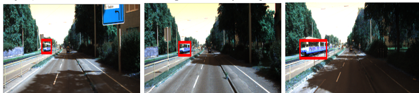
Labeling results from left to right: bus, car, train (ground truth). The object looks like a bus in the far field, but is classified as train when it's in the near field considering it's on railroad.
