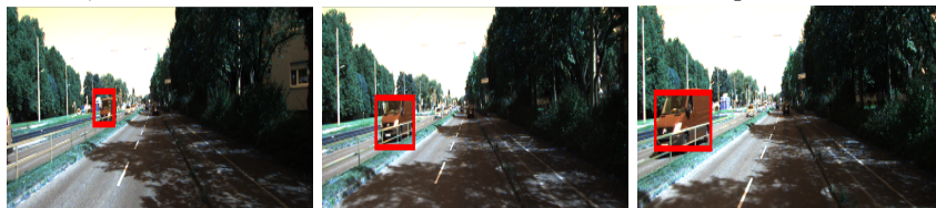
Labeling results from left to right: train, car, car (ground truth). The object looks like a train in the far field, but is classified as car when it's in the near field.
