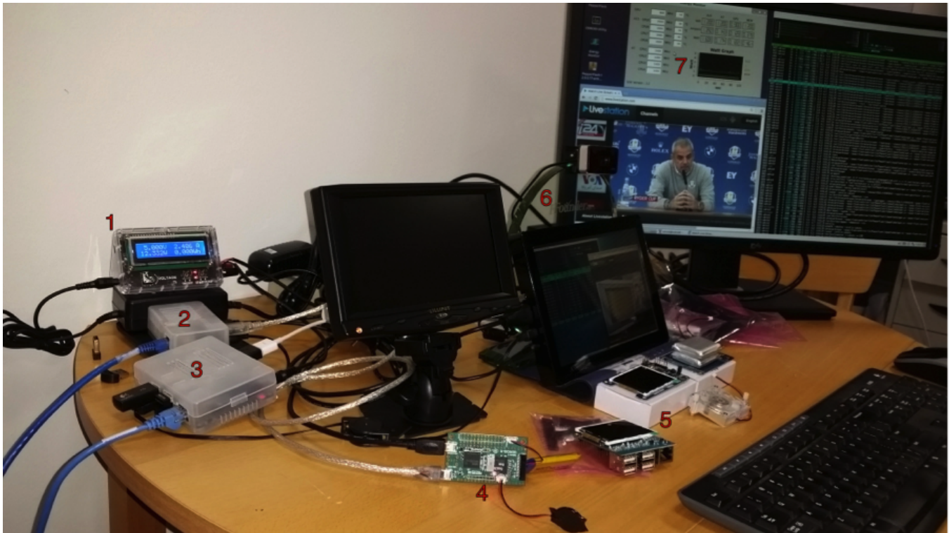
Figure 3.1: Some of the hardware devices benchmarked in this chapter are depicted above. Numbers superimposed on image correspond to: (1) Power meter indicating that three devices draw an aggregate of 12W at 5V. (2) Odroid U3, with case. (USB WiFi and Bluetooth dongles at left) (3) Odroid X-U3. (4) Odroid W (similar to Raspberry Pi). (5, 6 & 7) Assorted peripherals such as displays, various I/O ports, auxiliary fan, and battery pack.
