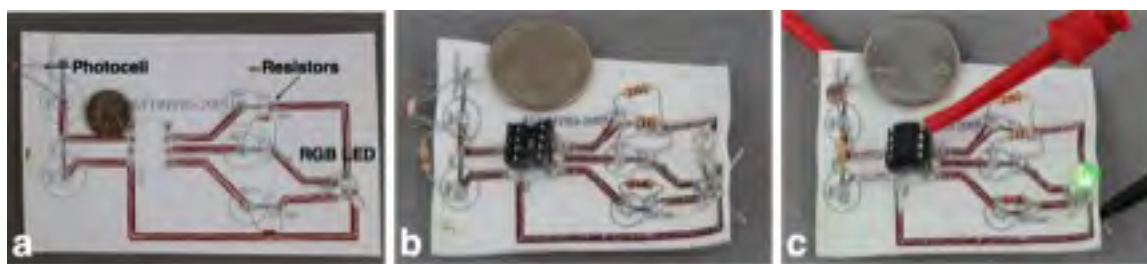
Figure 4.7: A ShrinkyCircuit designed using Eagle PCB software. a) Electronic components loaded on a circuit printed on polymer sheet with inkjet printer. The electrical connections are traced with a connective pen. c) IC holder is inserted into the shrunk circuit after the polymer substrate is heated. d) The ShrinkyCircuit under operation.
