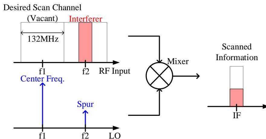
Figure 4.1: Reference spur issue in wavelet-based spectrum sensing.
