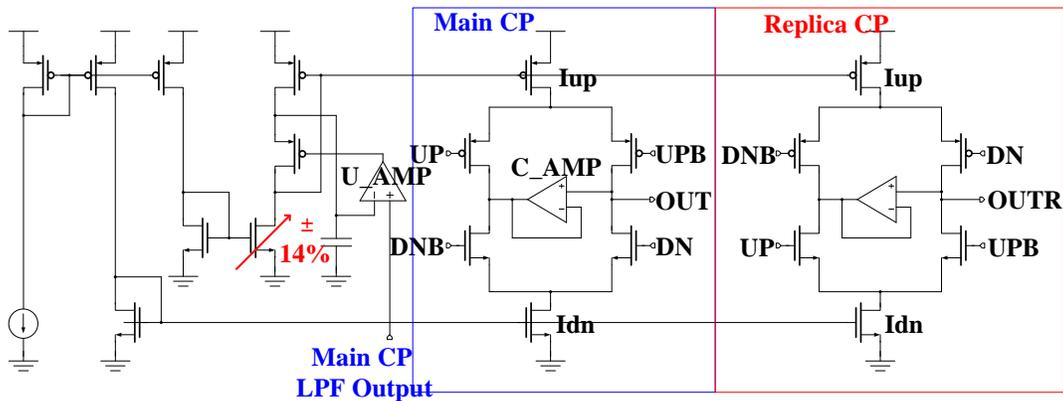
Figure 4.5: The proposed charge pump with the replica.
