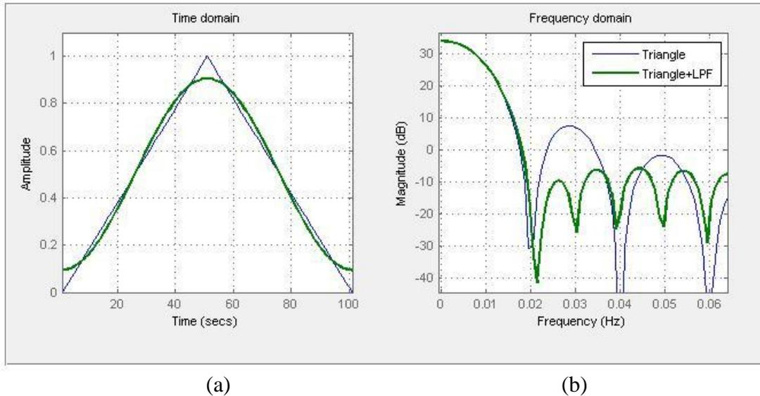
Figure 3.8: (a) Time domain plot and (b) power spectral densities of the triangular waveform without LPF and with 4<sup>th</sup> order Butterworth LPF
