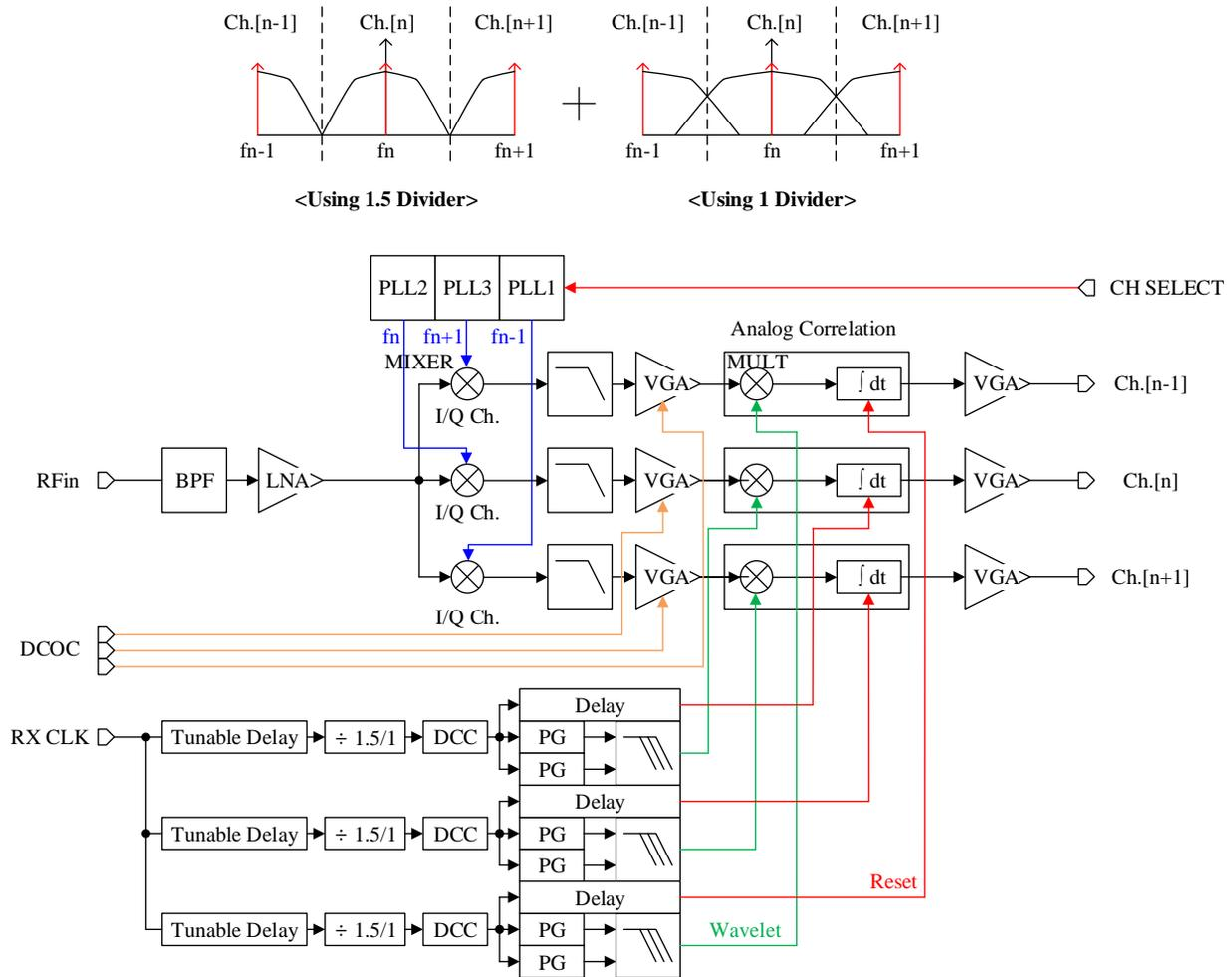
Figure 3.12: Proposed dual-resolution analog wavelet-based spectrum sensing
