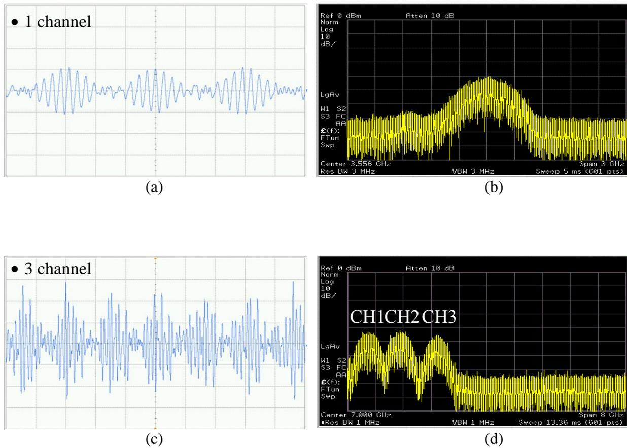
Figure 5.12: (a) Measured BPSK triangular-shaped pulse with a center frequency of 3.564GHz and (b) its power spectral density, and (c) measured BPSK triangular-shaped pulses with three center frequencies of 3.564GHz, 4.488GHz, and 5.412GHz and (d) their power spectral densities.
