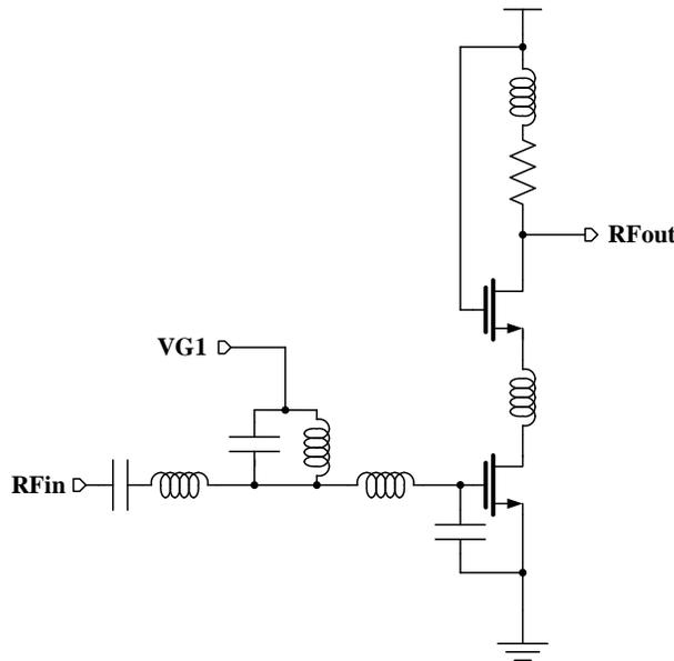
Figure 5.6: An ultra-wideband amplifier using Chebyshev active filter
