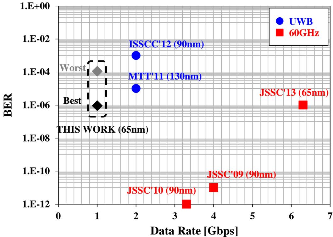
Figure 5.18: BER comparison with data rate and process
