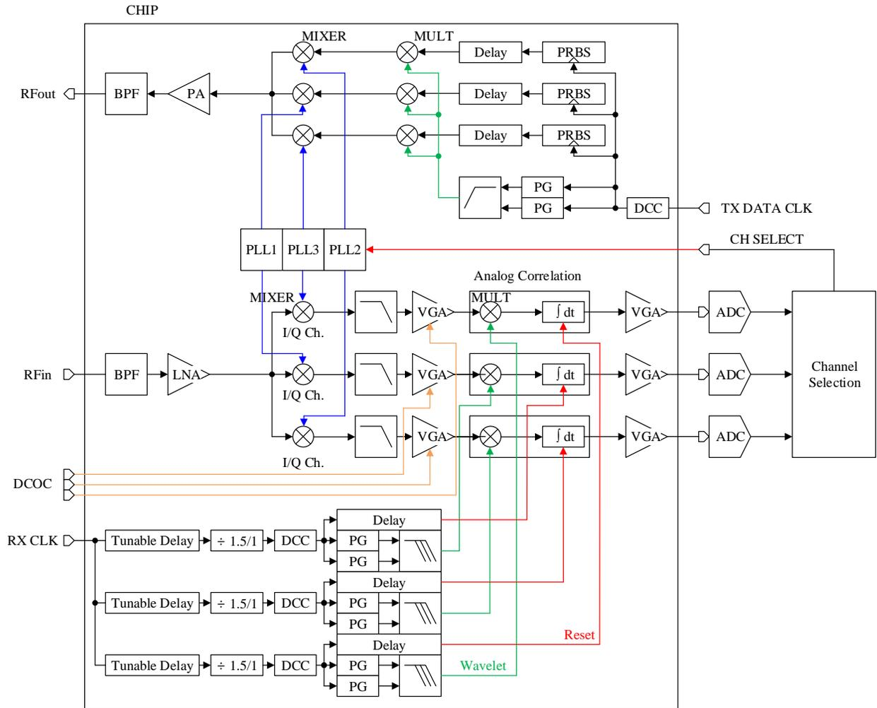
Figure 5.1: Architecture of Triple Channel UWB-based Cognitive IR-UWB
