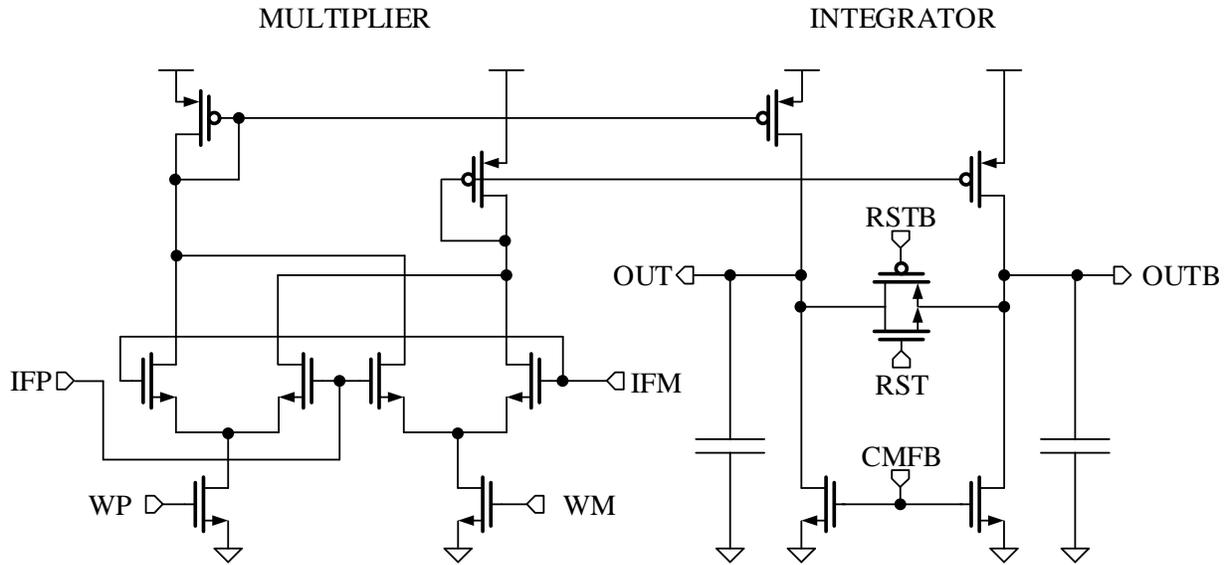
Figure 5.8: Gilbert-type analog correlation circuit with a multiplier and integrator.
