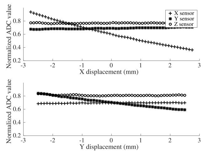
Figure 2.6: Sensor displacement test for three sensing elements. Top plot shows response of sensors to *x* displacement, and bottom plot shows response to *y* displacement, indicating that sensor responses are relatively independent.
