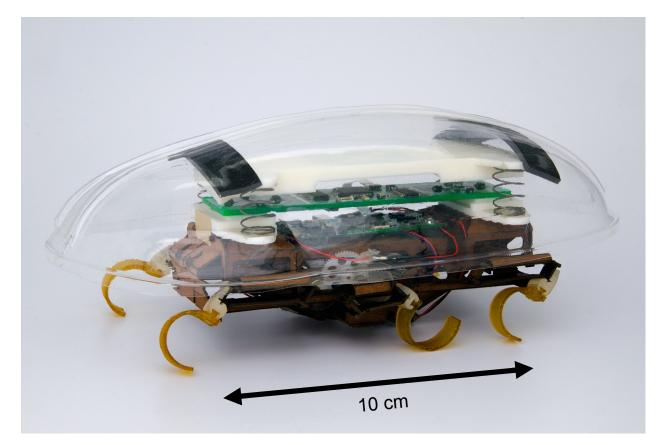
Figure 2.1: Force-torque sensor and shell mounted on a VelociRoACH.
