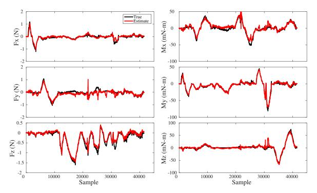
Figure 3.1: Comparison of true and estimated forces and torques for the test data set. True data was recorded using the commercial force-torque sensor and estimated data was calculated by applying the sensor response matrix to the SkinProc proximity sensor data.
