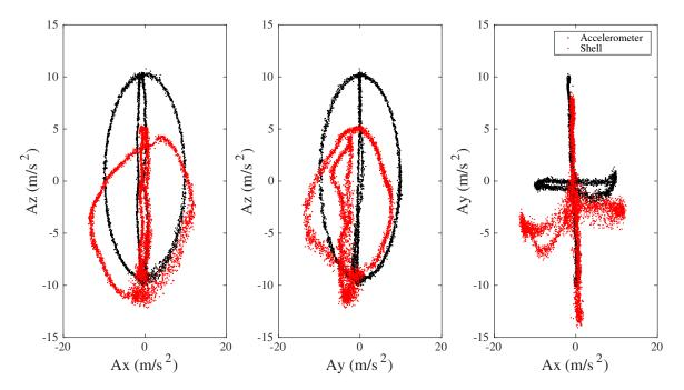
Figure 3.4: Slices of the three-dimensional acceleration vector space for the data from both the accelerometer and the shell through the rotation sequence of the robot.
