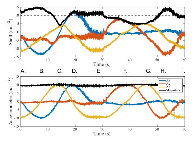
Figure 3.3: A comparison of the acceleration traces measured by both the shell and the accelerometer on board the VelociRoACH. The robot is slowly rotated first clockwise around its *y*-axis and then clockwise around its *x*-axis. Each letter marks a different orientation of the robot in the rotation sequence: A. legs down; B. nose up; C. legs up; D. nose down; E. legs down; F. left side down; G. legs up; H. left side up; I. legs down.
