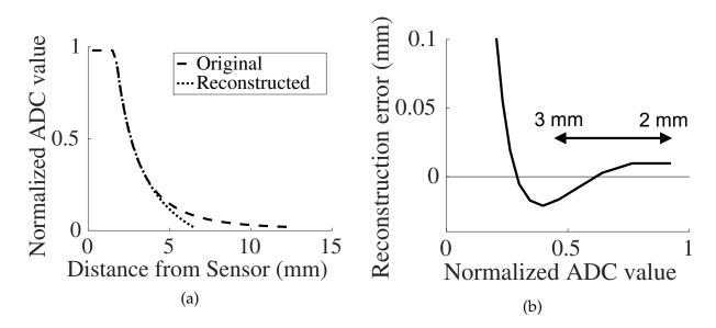
Figure 2.4: Response of individual sensor. (a) Proximity sensor response, and 1/r fit to curve. (b) Fitting error over 2-5 mm range, with error over most sensitive 2-3 mm range of less than 20  $\mu$ m.
