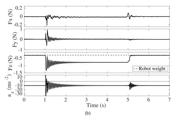
Figure 3.5: Step response of sensor to a 50 gram mass. (a) Photo of VelociRoACH on its back with a 50 gram mass resting on its underside. (b) Three-axis force data and *z*-axis accelerometer data for a 50 gram mass placed on the robot at 1 second and removed at 5 seconds.
