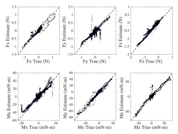
Figure 3.2: Measured and reconstructed force-torque data compared directly. Time is eliminated in order to visualize the linearity of the mapping over a range of forces and torques. The dashed lines have slopes of 1, indicating an ideal 1-to-1 linear mapping.
