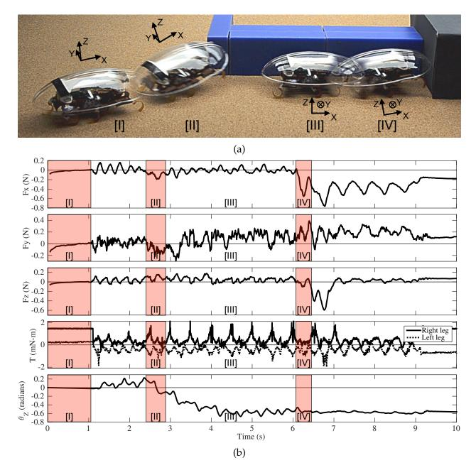
Figure 3.6: The VelociRoACH in (a) is shown stationary [I], running into a corner [II], following a wall [III], and colliding with a perpendicular wall [IV]. The corresponding x, y, and z forces, as well as the right and left leg torques and the integrated z-axis gyroscope data are shown in (b).
