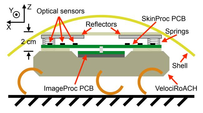
Figure 2.2: Side view of sensor and shell mounted on a VelociRoACH, showing optical proximity sensors and sensing springs.
