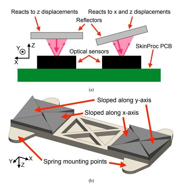
Figure 2.5: Principle of operation of force-torque sensor. (a) Spring supported reflective element has sloped reflector geometry that responds to lateral and normal displacement. (b) Complete floating reflective element with 4 reflectors at each end, corresponding to each of 8 proximity sensors.
