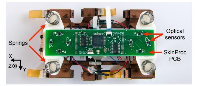
Figure 2.3: Photo showing custom SkinProc sensing board with 8 proximity sensors mounted in two arrays.
