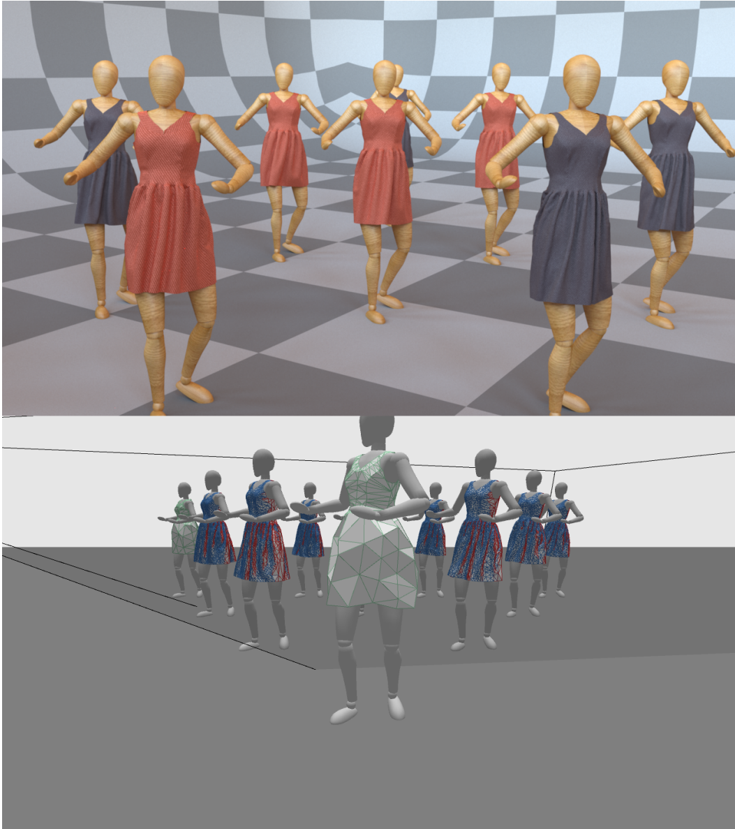
Figure 7: A group of multiple dancers is rendered from the camera's perspective (top), while an external view showing the camera's view frustum is shown below. Characters completely outside the view frustum are simulated at very low resolution.
