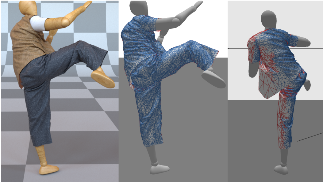
Figure 1: The clothing on this character uses view-dependent simulation. Visible areas (blue) are simulated at high resolution, as measured in screen-space. Areas not visible to the camera (red) are simulated at reduced resolution. The first two images show views from the camera’s perspective. The rightmost image shows an outside perspective with the camera’s view frustum drawn in black wireframe.
