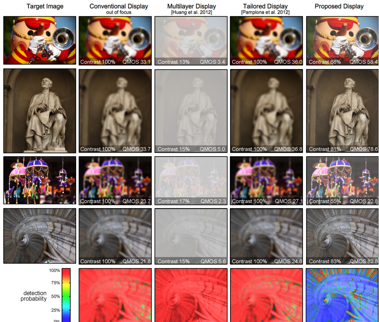
Figure 4.2: Evaluation of vision-correcting displays. We compare simulations both qualitatively and quantitatively using contrast and quality-mean-opinion-square (QMOS) error metrics. A conventional out-of-focus display always appears blurred (second column). Multilayer displays with prefiltering improve image sharpness but at a much lower contrast (third column). Light field displays without prefiltering require high angular resolutions, hence provide a low spatial resolution (fourth column). The proposed method combines prefiltering and light field display to optimize image contrast and sharpness (right column). The QMOS error metric is a perceptually linear metric, predicting perceived quality for a human observer. We also plot maps that illustrate the probability of an observer detecting the difference of a displayed image to the target image (bottom row). Our method performs best in most cases. (Source images courtesy of flickr users Jameziecakes, KarHan Tan, Mostaque Chowdhury, Thomas Quine (from top)) This figure is from [5].
