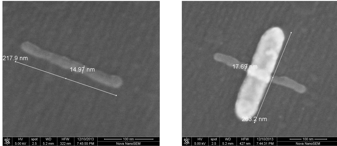
Figure 39. Completed fabrication of a) bare InP ridge and b) optical antenna device before substrate removal
