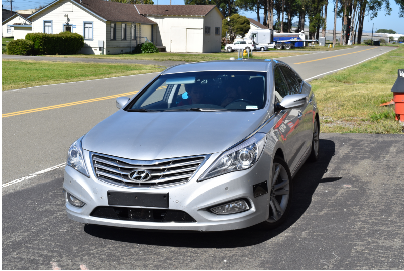
Figure 1-1: The prototype test vehicle was a Hyundai Grandeur. It is equipped with a camera, GPS/INS system, six laser rangefinders, and radar sensors.
