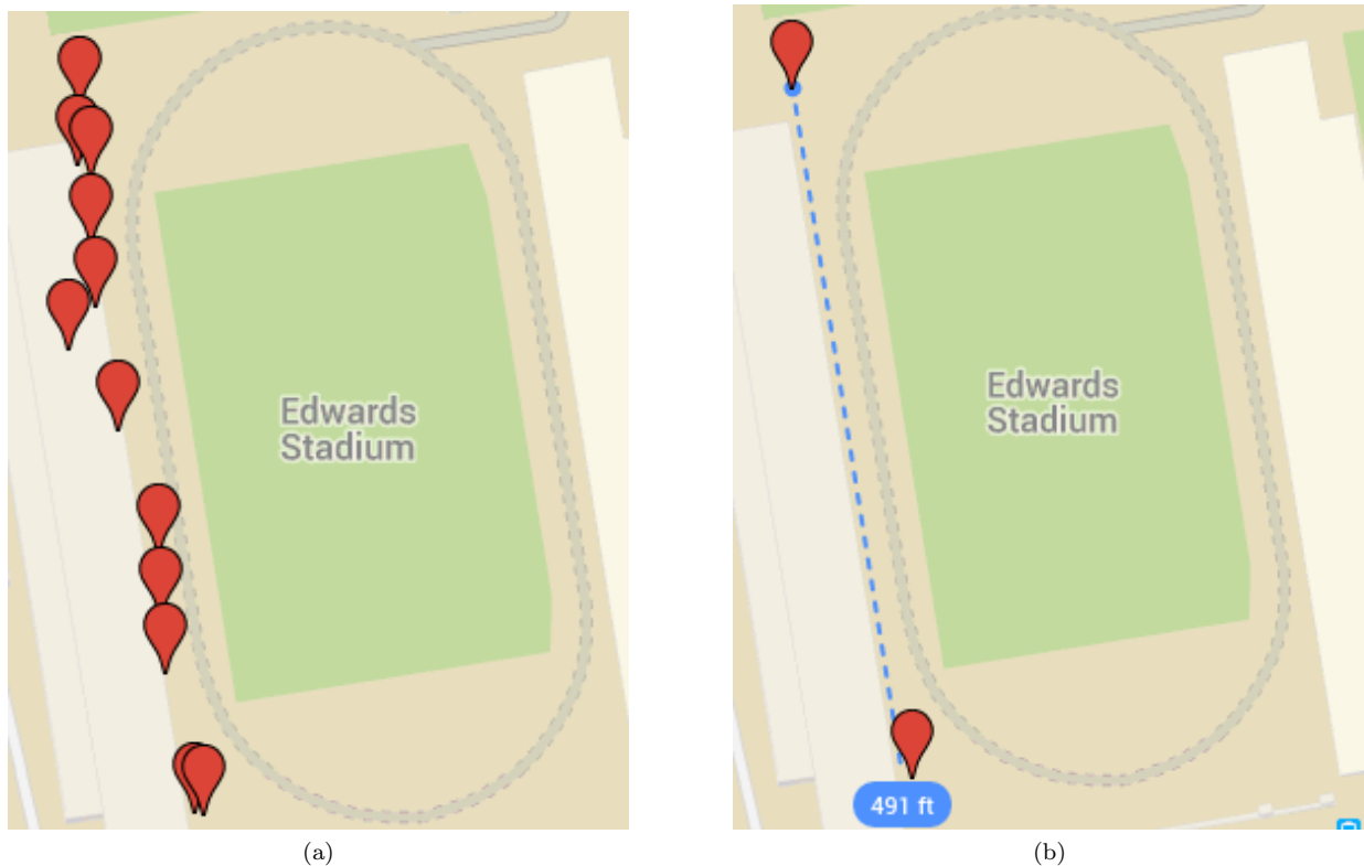
Figure 1.6: (a) Google Maps Plot of Collected GPS Datapoints (b) Google Maps Distance Measurement of Start to End Coordinates
