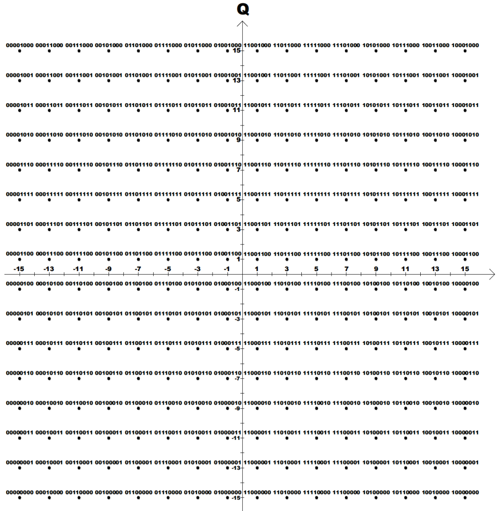
Figure 4: bit encoding for 256-QAM as an extension to IEEE 802.11a. (Yeh & Seo 2007:6)
