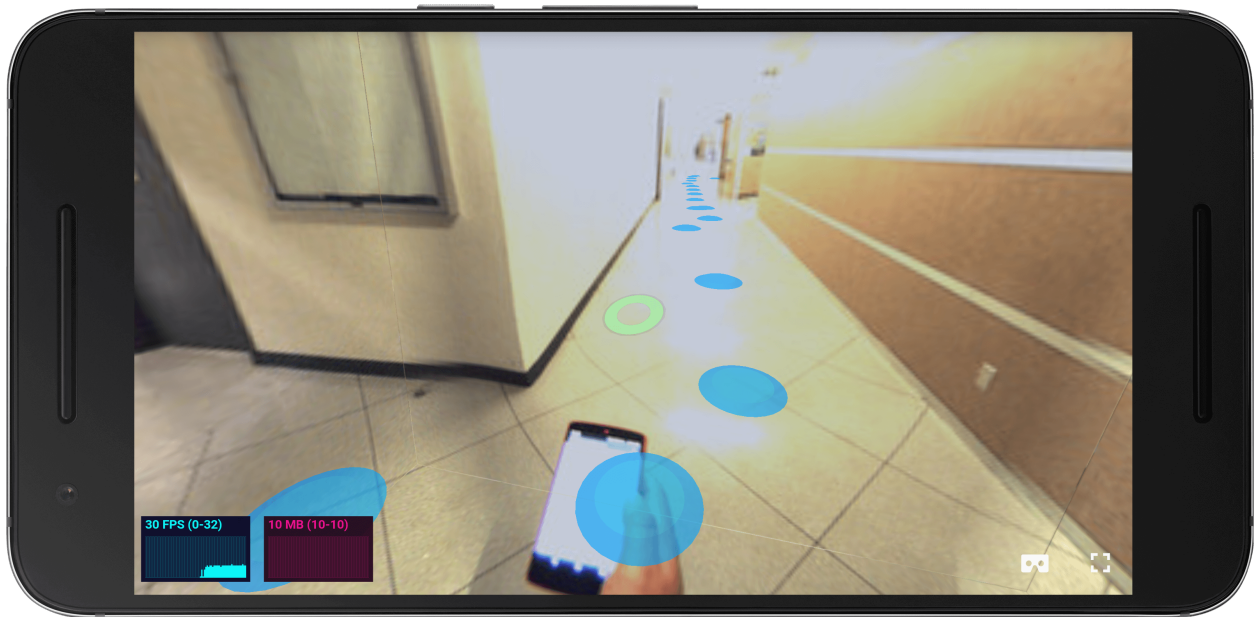
Figure 3.1: The final system in Fullscreen Mode. The green circle in the middle is the pancake, located where the user is pointing the controller.
