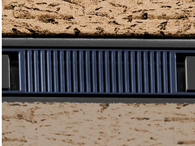
Figure 4.23 Close-up SEM image of released HCG reflector before actuation.
