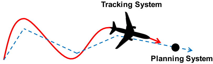
Figure 5.7: A planning system using a fast but simple model, followed by a tracking system using a dynamic model
