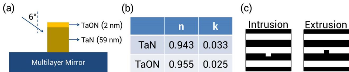
Figure 3.9: (a) Side view of a schematic diagram of EUV mask pattern: absorber pattern height and illumination orientation. (b) Optical properties of the absorber materials at EUV wavelength (13.5 nm). (c) Top-down view of intrusion / extrusion defect definition: Black is the absorber and white is the spacing.
