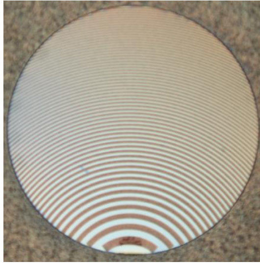
Figure 5.12: SEM image of a standard off-axis zoneplate used by the SHARP EUV microscope. The diameter of the zoneplate is around 100 \mu\text{m} .
