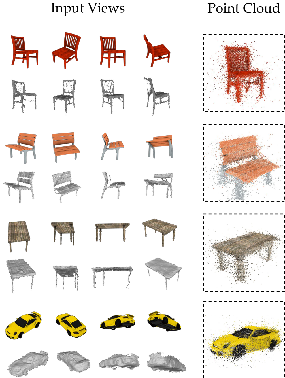
Figure 4.5: Qualitative results for per-view depth map prediction on ShapeNet. We show the depth maps predicted by Depth-LSM (visualized with shading from a shifted viewpoint) and the point cloud obtained by unprojecting them into world coordinates.
