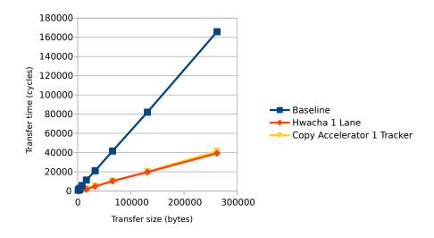
Figure 5: Baremetal memcpy() performance
