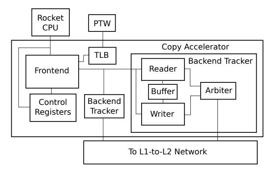
Figure 3: Accelerator Design
