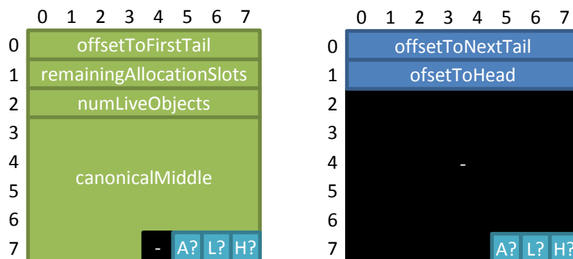
Figure 4.2: Oscar++ metadata for head (left) and tail (right) objects. A = truly aliased (see Section 4.2.3), L = live object, H = head.
