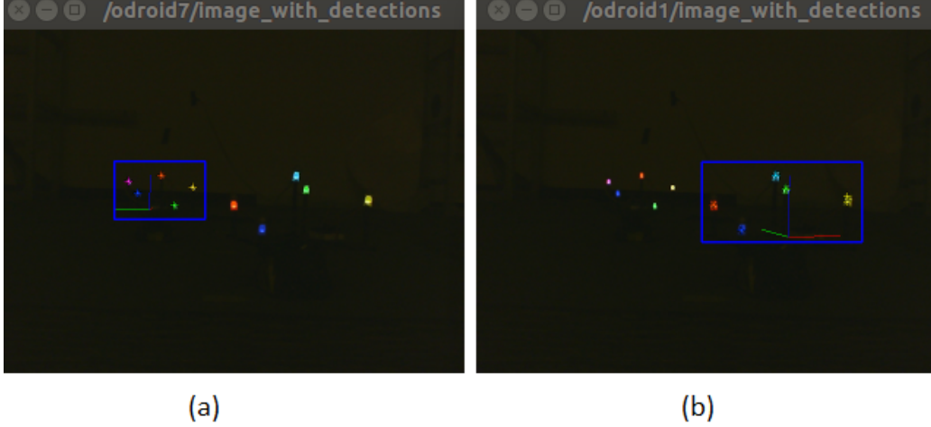
Figure 5: Example frame of relative pose estimation. Picket-1’s pose tracker is in (a) and picket-2’s pose tracker is in (b). Picket-1 and picket-2 share four colors respectively. The bounding boxes shown in blue correspond to the area where the pose estimator is searching for LEDs. LEDs associate are marked with a crosshair of their respective color on the associated pose estimator. The body frame of the picket robots are overlaid with the convention RGB-XYZ.
