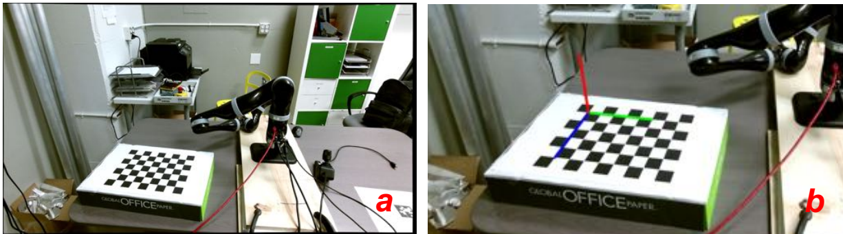
Image 9, Image of checkerboard pattern on lab table. (a) an example of input image to the extrinsic calibration node. (b) after extrinsic calibration, the node is able to detect the x , y , z axis and draw them on the image.
