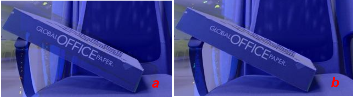
Image 8, overlay of IR and RGB images before and after calibration. (a) before calibration, there is a shallow IR “shadow” of the box to the right of its color image. (b) after calibration, the “shadow” overlaps completely with its color image.
