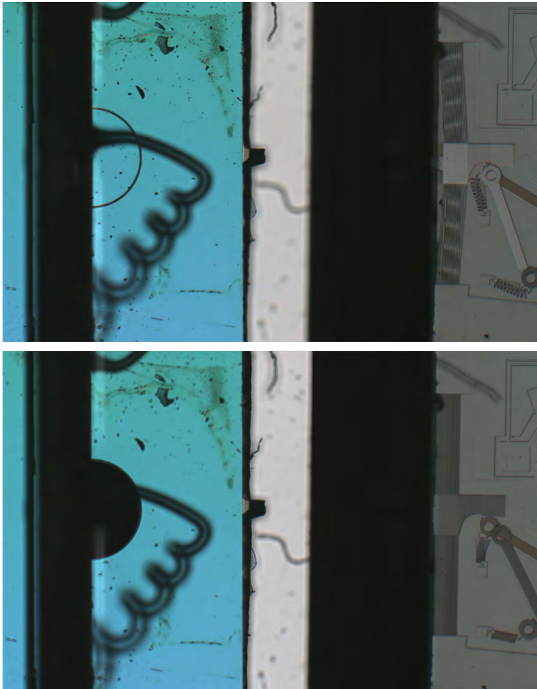
Figure 2.23: Before (top) and after (bottom) images of the electrically initiated fracture of a membrane. In both images, the left side of the image shows the physical chips and right right side shows the hammer chip as seen through the 45 degree mirror.
