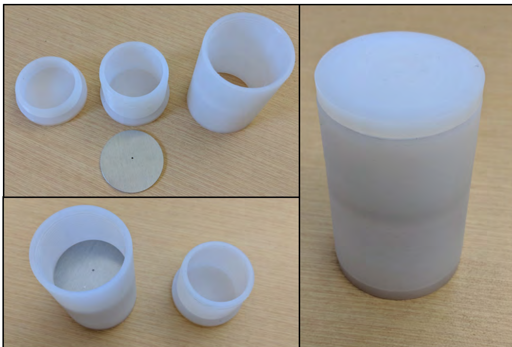
Figure 2.1: The PFA package used to house the XeF_2 and MEMS components.
