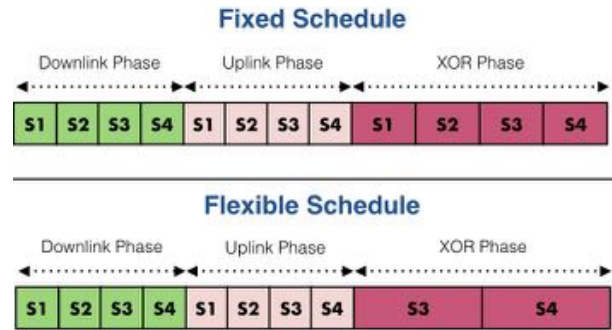
(b) Fixed and flexible scheduling for the star topology example considered in Fig. 3.15. The green boxes correspond to the downlink packets from the controller to the client nodes (the destinations are labelled: S_i ). The pink boxes correspond to the uplink packets from the client nodes to the controller (the origins are labelled). The purple boxes correspond to the XOR packets where the label corresponds to client node whose DL and UL packets are XORed.
