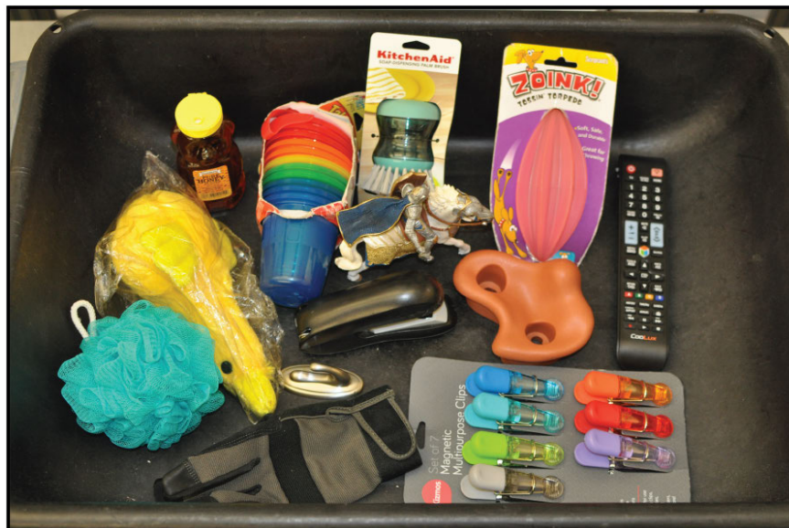
Figure 8.10: Several objects that cause failures across composite policies that plan grasps for suction and parallel-jaw grippers based on point cloud geometry alone.
