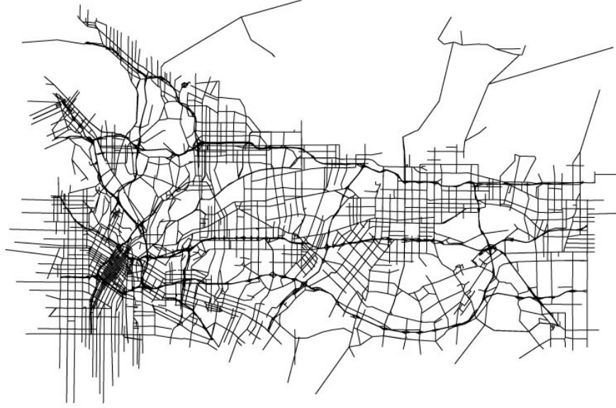
Figure 35: Full-scale network including highway and arterial networks of the I-210 corridor used for MATSim data generation, and for the estimation problem. See Figure 31 for the Voronoi tessellation model of the cellular network and the 700 origins given by the TAZ.
