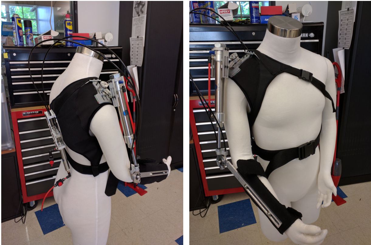
Figure 8.10: APEX- \gamma . Left: Side view showing the refined backplate, and shoulder harness. Right: Front view showing the elbow mechanism and arm brace.
