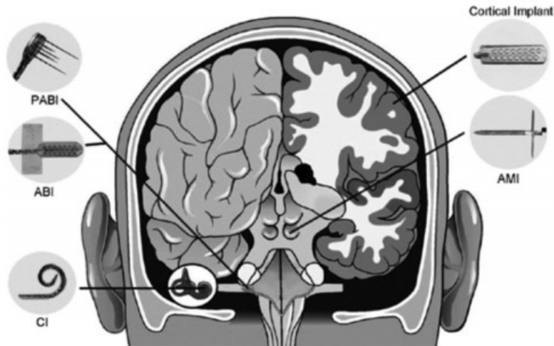
Figure 1-6: Implants using DBS to treat tinnitus and restore hearing [JOH]
