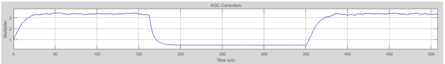
Figure 6.3.2: AGC Correction During Frame Reception (No Carrier or Timing Frequency Offset)
