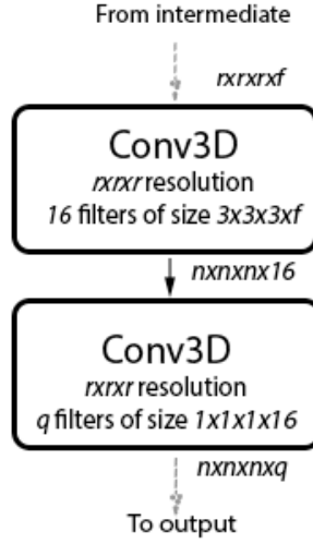
Fig. 4: A hook layer consisting of two 3D convolution operations, used in Figure 1. q is n_{classes} + 1 for a classification hook output and 7 for a localization hook output.
