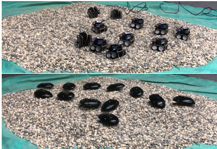
Figure 4.1: Over 15 teleoperated trials performed on rough terrain, a legged robot succeeded in navigating through the terrain 90% of the time, whereas a tracked robot of comparable size succeeded only 30% of the time.
