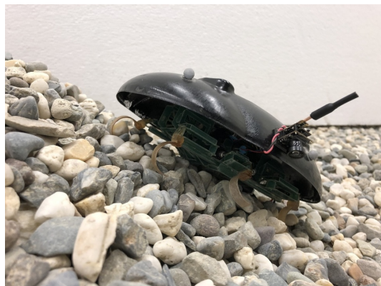
Figure 1.1: VelociRoACH: the small, mobile, highly dynamic, and bio-inspired hexapedal millirobot used in this work, shown with a camera mounted for terrain imaging.
