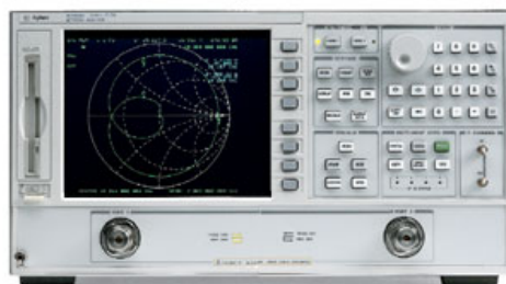
Figure 2.6: An HP 8722D VNA used for FMR measurements. The 8722D has a frequency range of 50 MHz to 40 GHz, and can output signals with a power of -5 dBm up to 20 GHz, or -10 dBm up to 40 GHz. The SMA connectors used in this setup limit the maximum frequency to 25 GHz, however.
